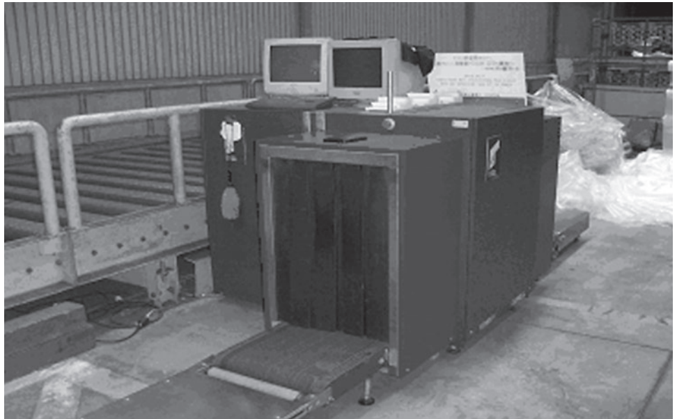
Figure 2: Type of X-ray Technology Used by Some Foreign Air Carriers to Inspect Air Cargo Bound for the United States
