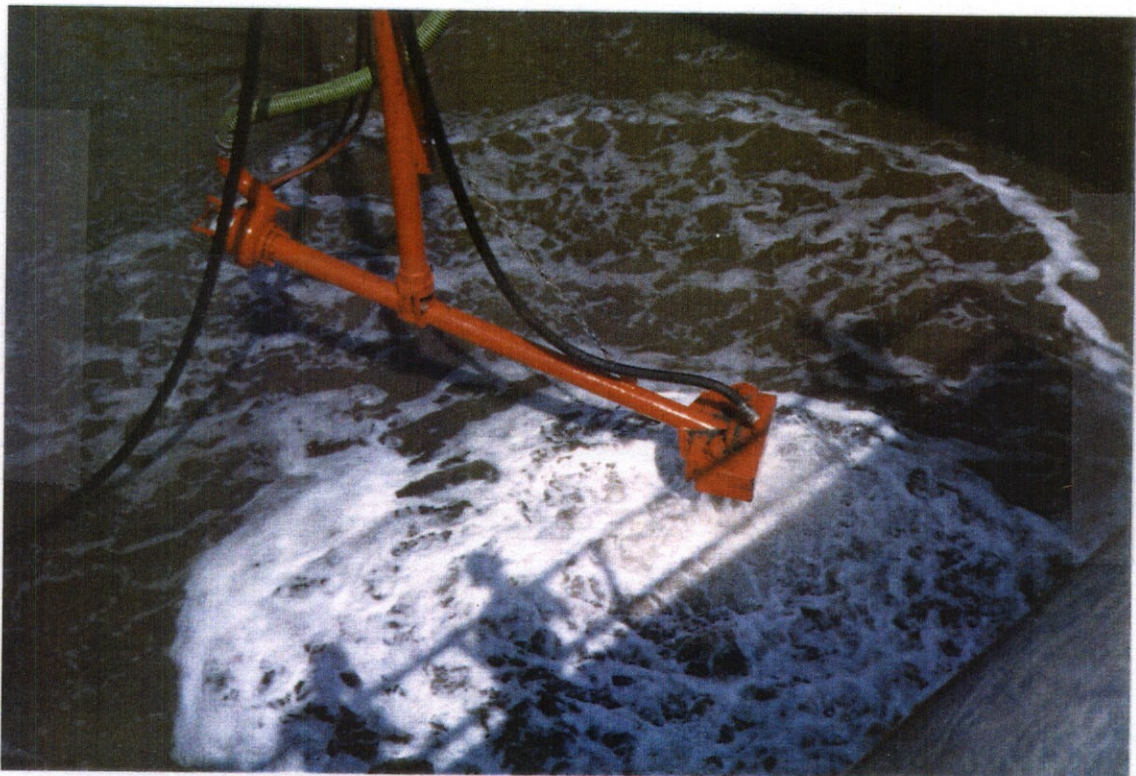
JET DREDGE SHOWING THE ACTION OF THE LANCING JETS
