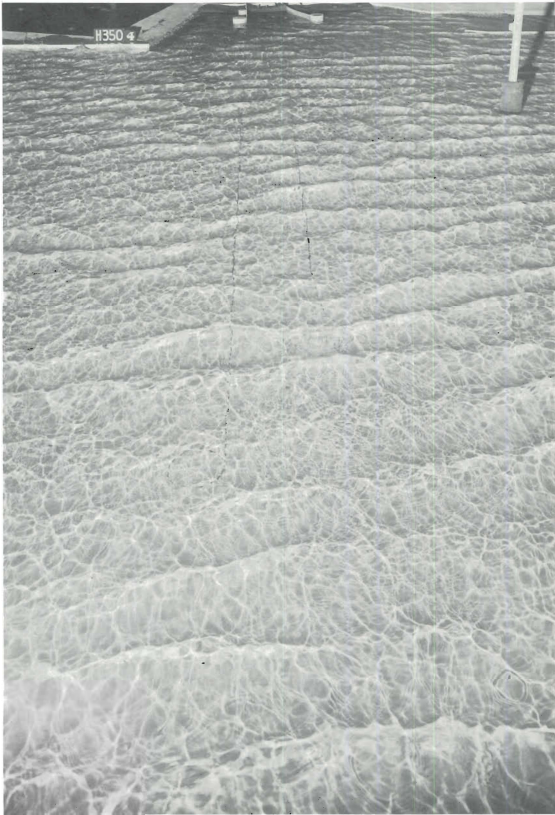
Photo 4. Typical wave patterns for existing conditions; 4-sec, 4-ft waves from NNW; swl = +1 ft msl
