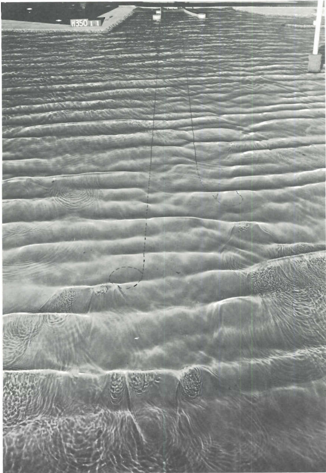
Photo 10. Typical wave patterns for Plan 1; 3-sec, 4-ft waves from NNW; swl = +1 ft msl
