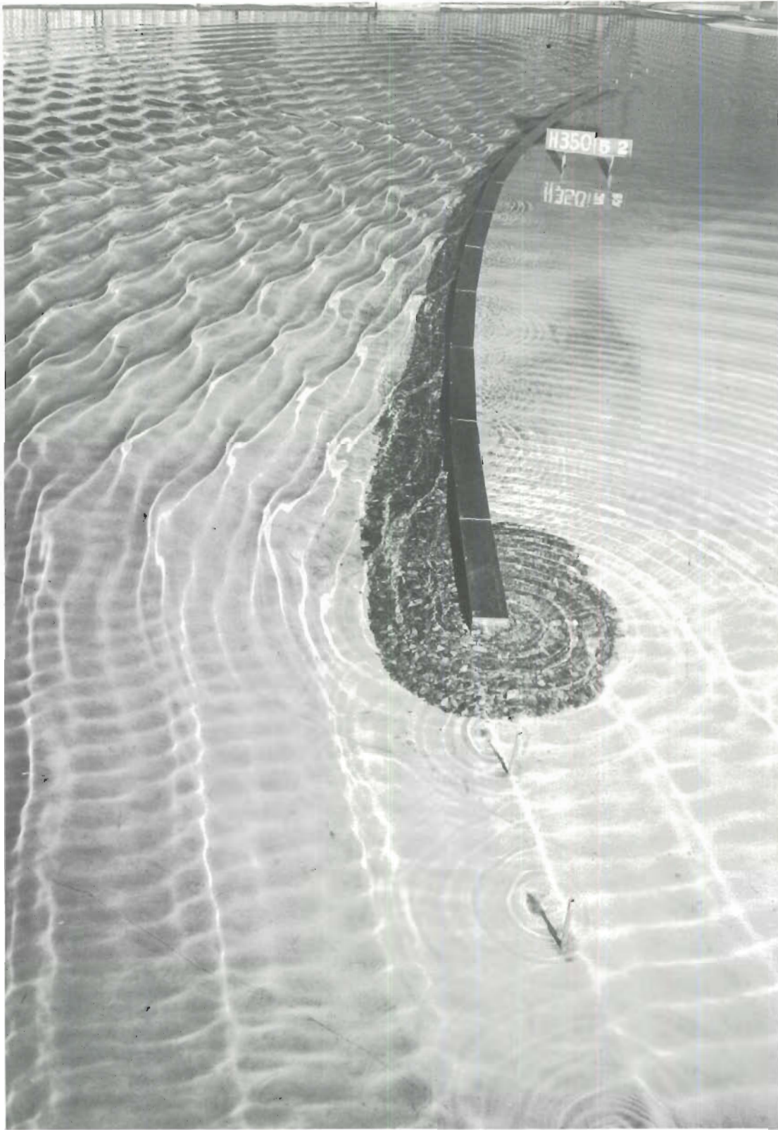
Photo 64. Typical wave patterns at breakwater for Plan 12A; 4-sec, 4-ft waves from NW; swl = +1 ft msl
