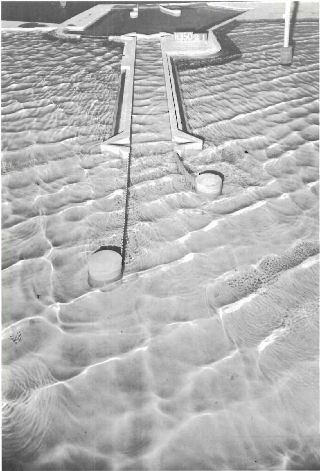
Photo 19. Typical wave patterns at lock entrance for Plan 2; 3-sec, 4-ft waves from NW; swl = +1 ft msl
