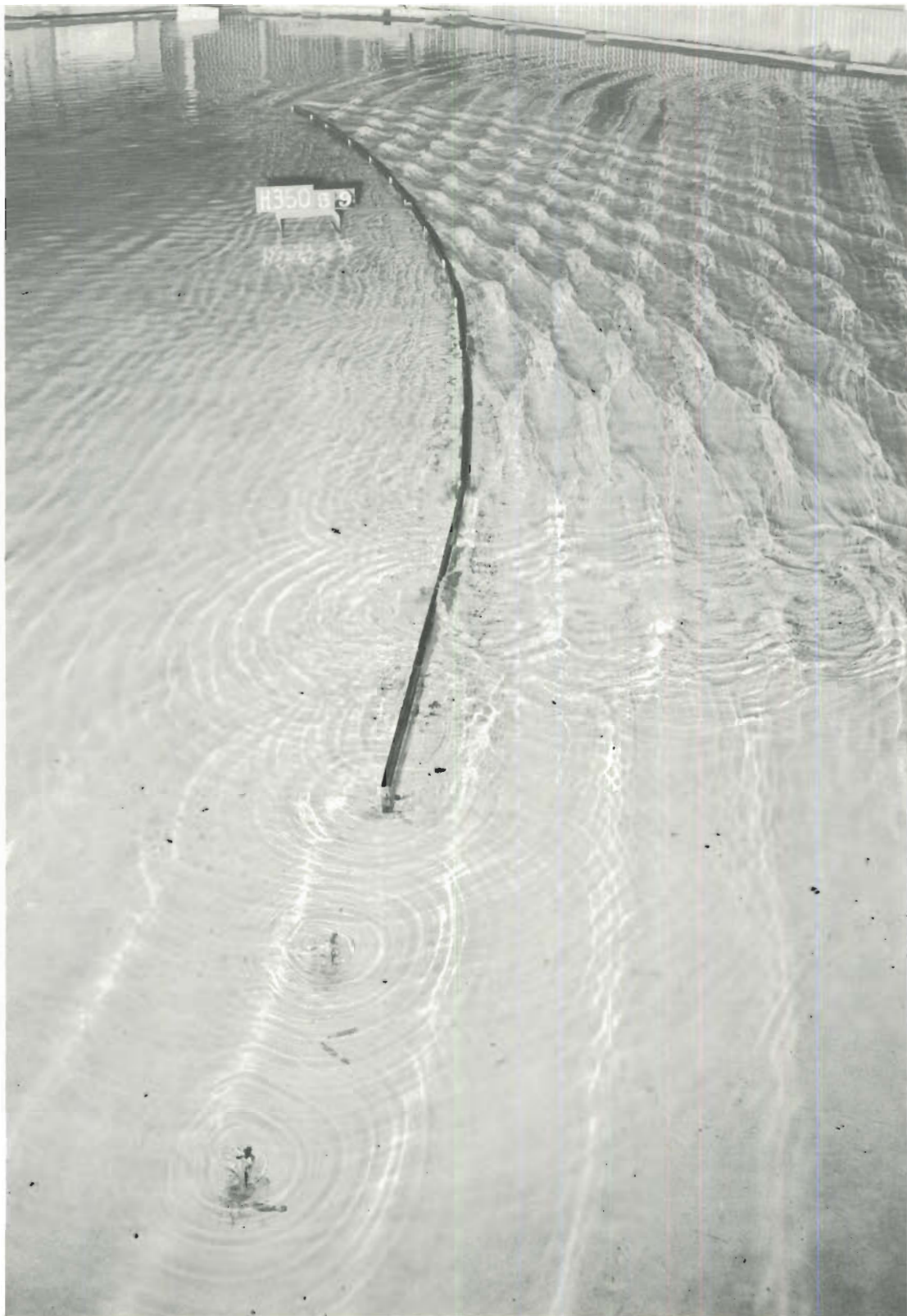
Photo 56. Typical wave patterns at breakwater for Plan 11B; 4-sec, 5-ft waves from N; swl = +1 ft msl
