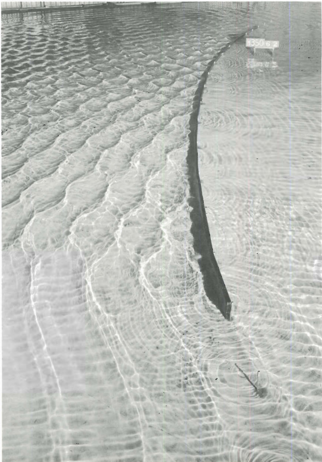
Photo 58. Typical wave patterns at breakwater for Plan 11B; 4-sec, 4-ft waves from NW; swl = +1 ft msl
