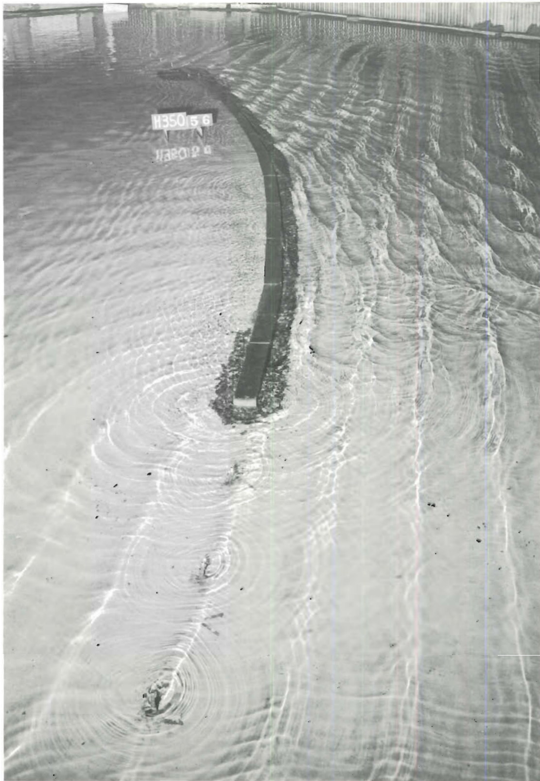
Photo 62. Typical wave patterns at breakwater for Plan 12A; 4-sec, 5-ft waves from N; swl = +1 ft msl
