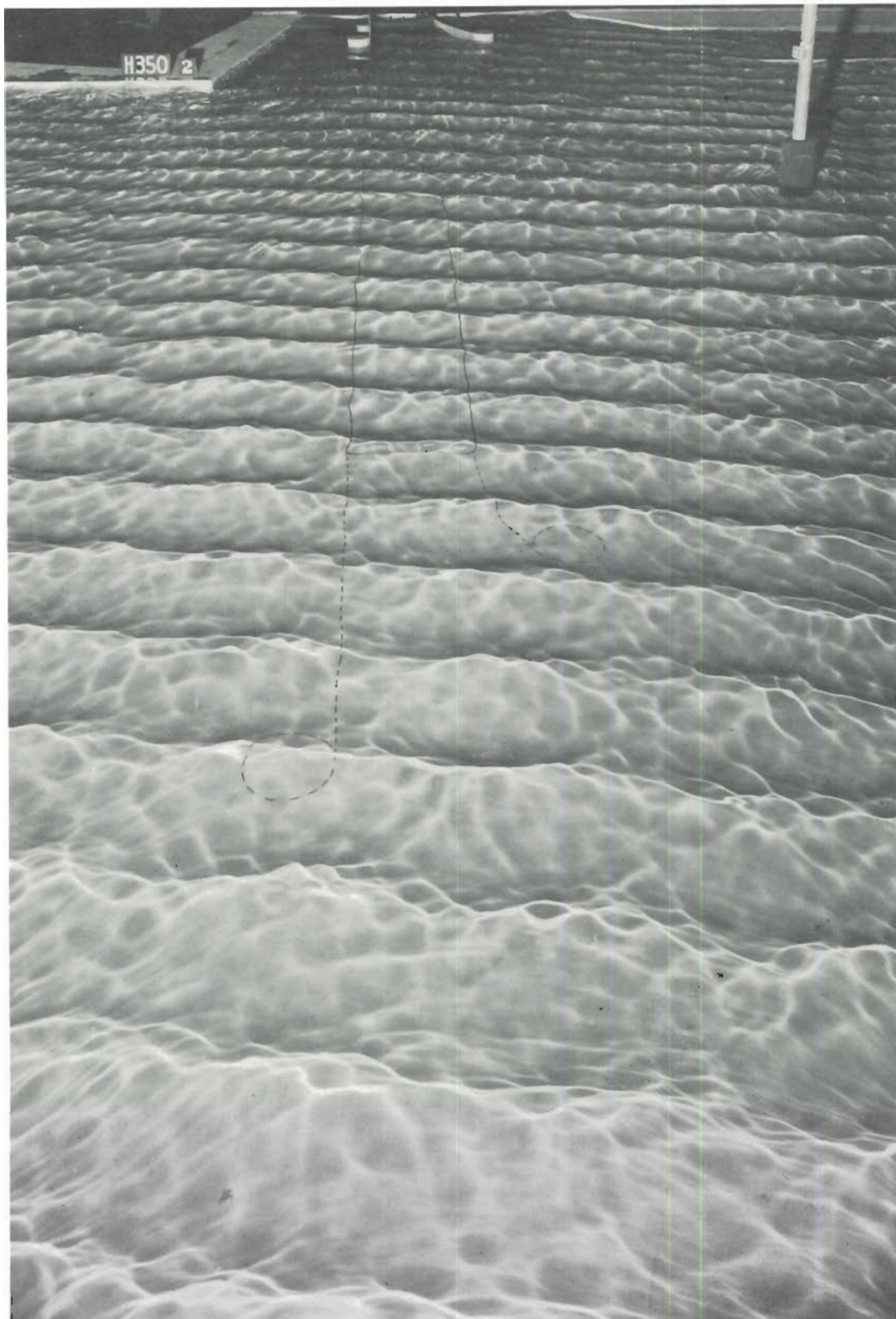
Photo 2. Typical wave patterns for existing conditions; 4-sec, 5-ft waves from N; swl = +1 ft msl
