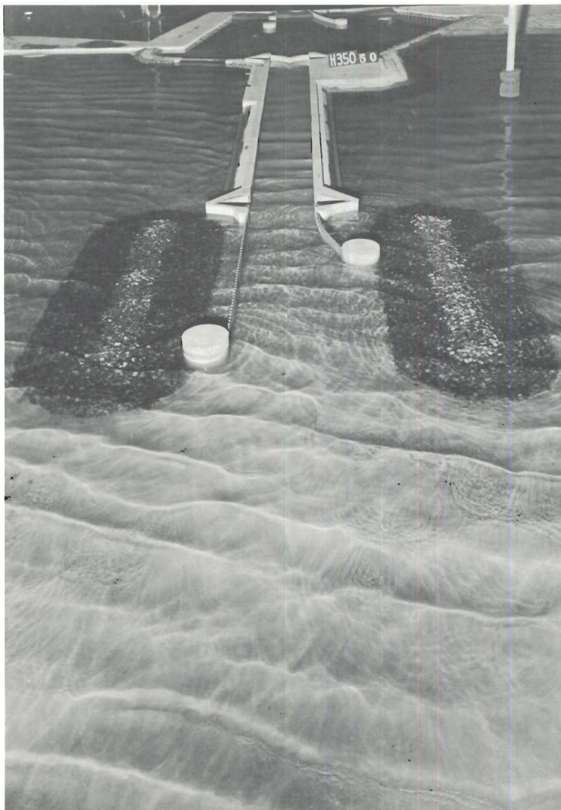
Photo 42. Typical wave patterns at lock entrance for Plan 9; 3-sec, 4-ft waves from N; swl = +1 ft msl
