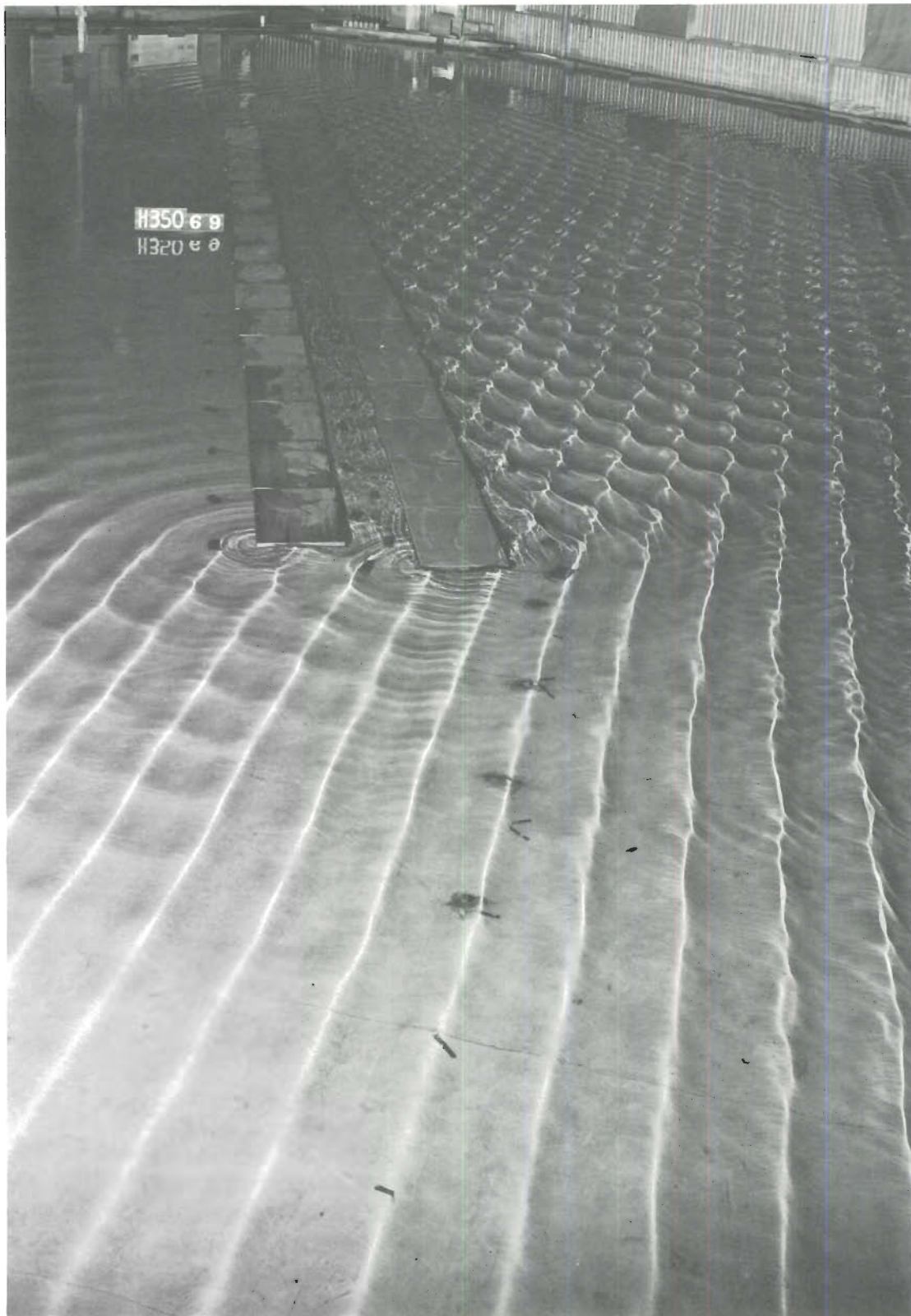
Photo 68. Typical wave patterns at breakwater for Plan 17C; 3-sec, 4-ft waves from N; swl = +1 ft msl
