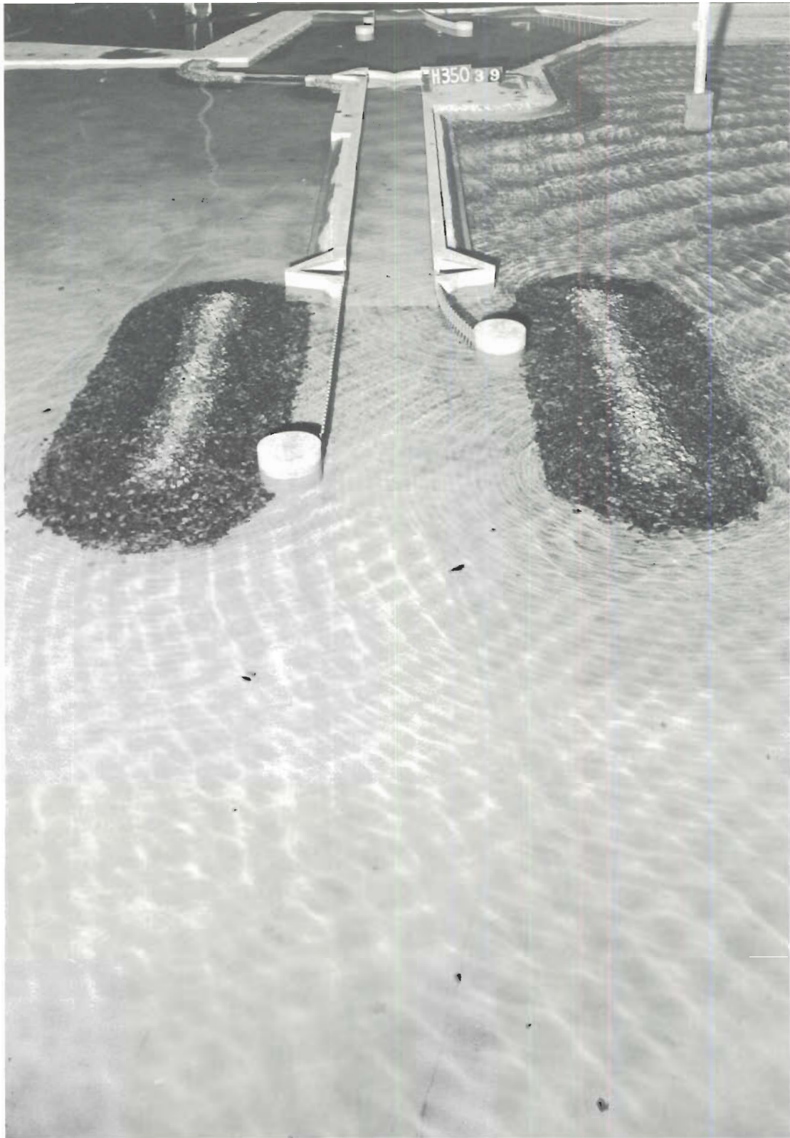
Photo 38. Typical wave patterns at lock entrance for Plan 8; 4-sec, 4-ft waves from NW; swl = +1 ft msl
