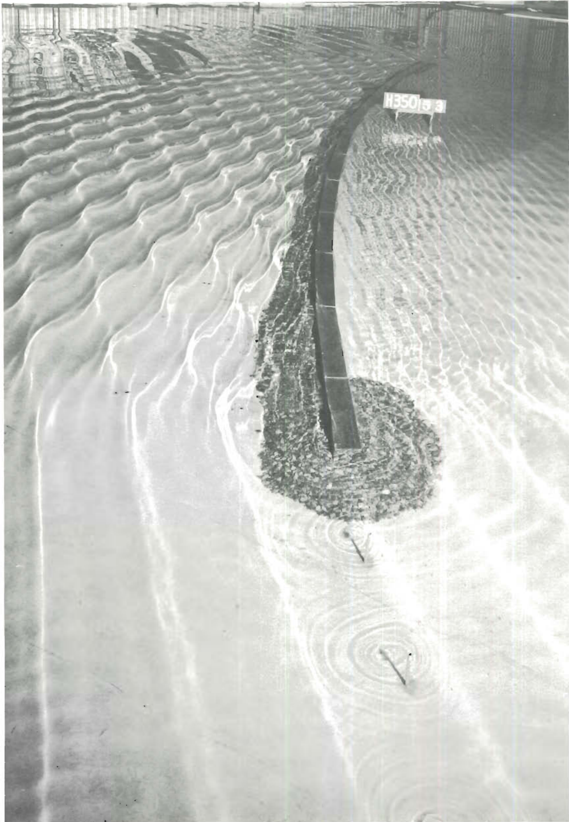
Photo 66. Typical wave patterns at breakwater for Plan 12A; 4-sec, 4-ft waves from NW; swl = +4 ft msl
