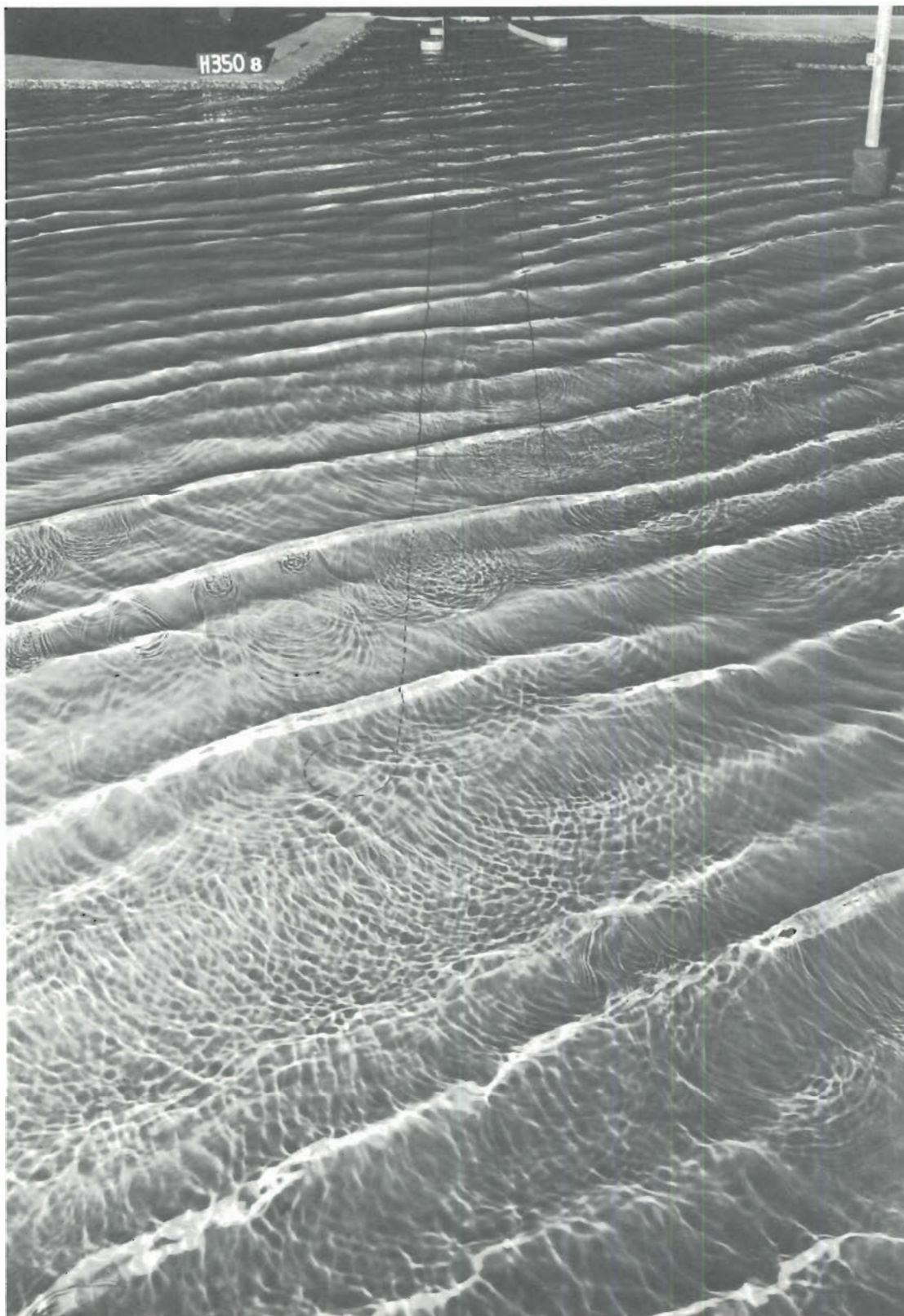
Photo 12. Typical wave patterns for Plan 1; 3-sec, 4-ft waves from NW; swl = +1 ft msl
