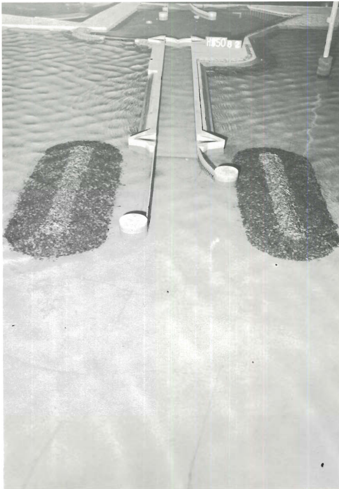
Photo 82. Typical wave patterns at lock entrance for Plan 20A; 3-sec, 4-ft waves from NNW; swl = +1 ft msl
