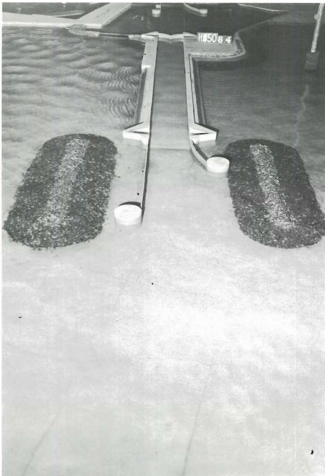
Photo 81. Typical wave patterns at lock entrance for Plan 20A; 4-sec, 5-ft waves from N; swl = +1 ft msl
