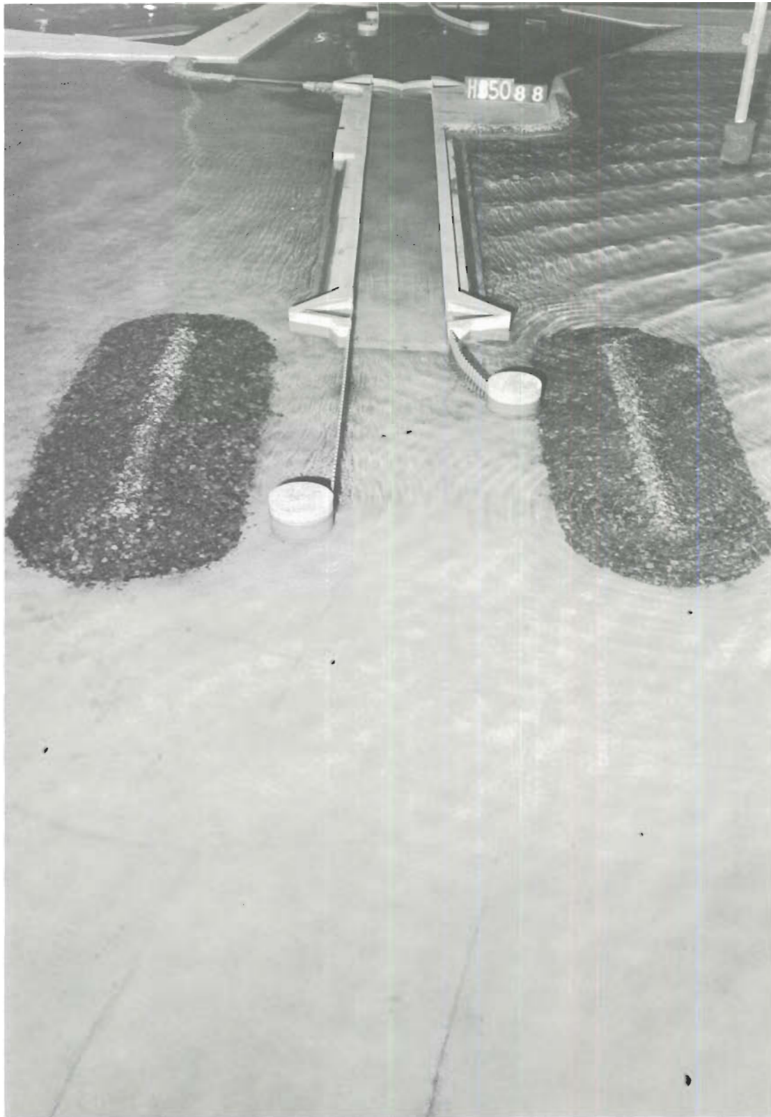
Photo 86. Typical wave patterns at lock entrance for Plan 20A; 4-sec, 4-ft waves from NW; swl = +4 ft msl
