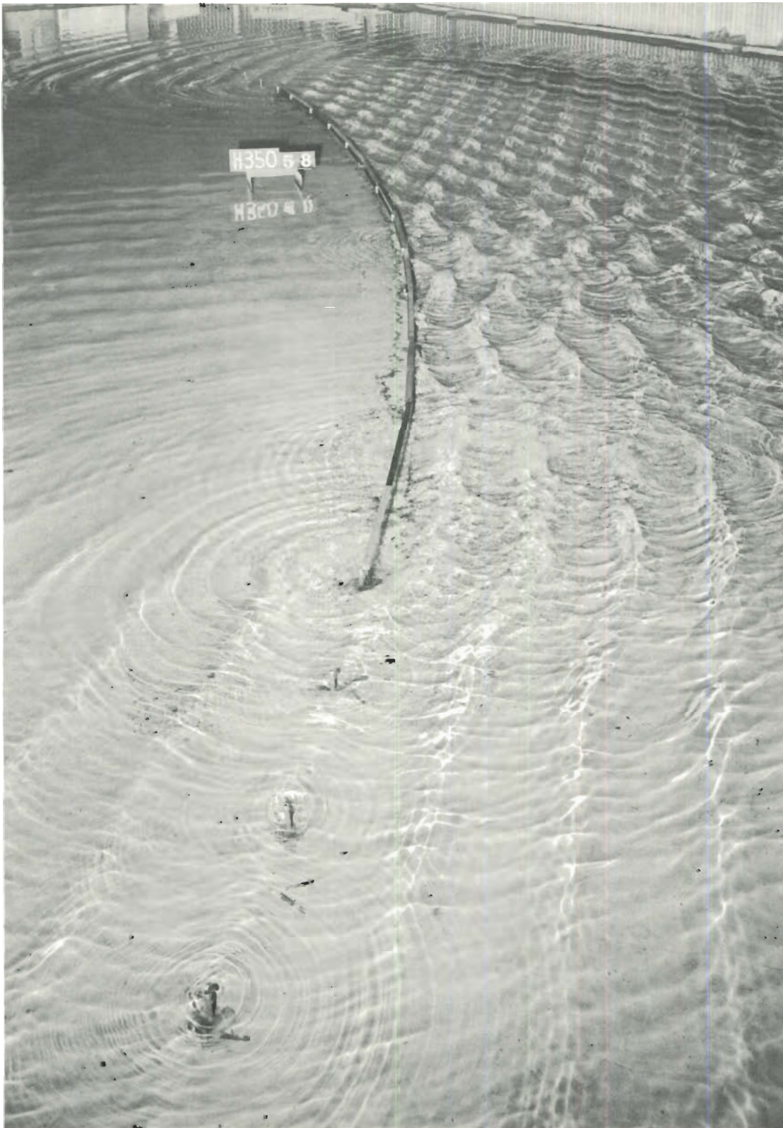
Photo 50. Typical wave patterns at breakwater for Plan 10A; 4-sec, 5-ft waves from N; swl = +1 ft msl
