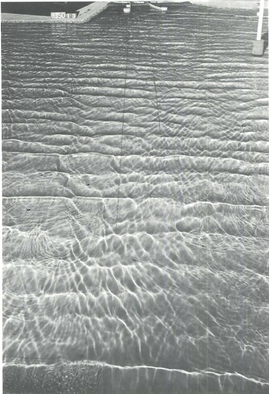
Photo 8. Typical wave patterns for Plan 1; 3-sec, 4-ft waves from N; swl = +1 ft msl
