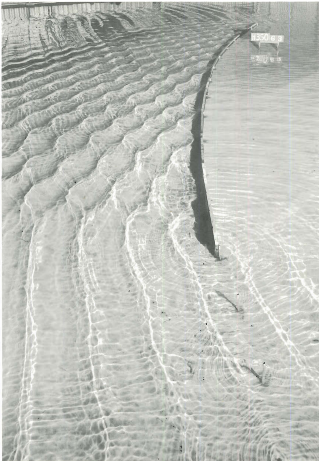
Photo 52. Typical wave patterns at breakwater for Plan 10A; 4-sec, 4-ft waves from NW; swl = +1 ft msl
