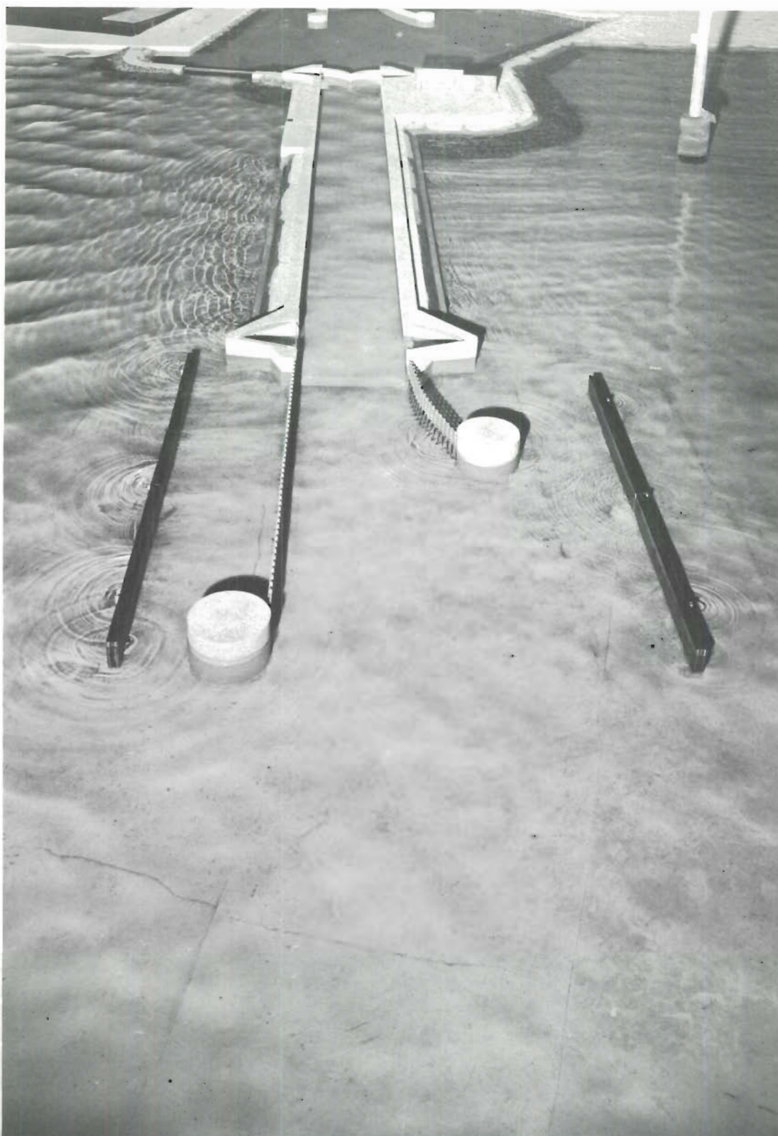
Photo 77. Typical wave patterns at lock entrance for Plan 19F; 4-sec, 5-ft waves from N; swl = +1 ft msl
