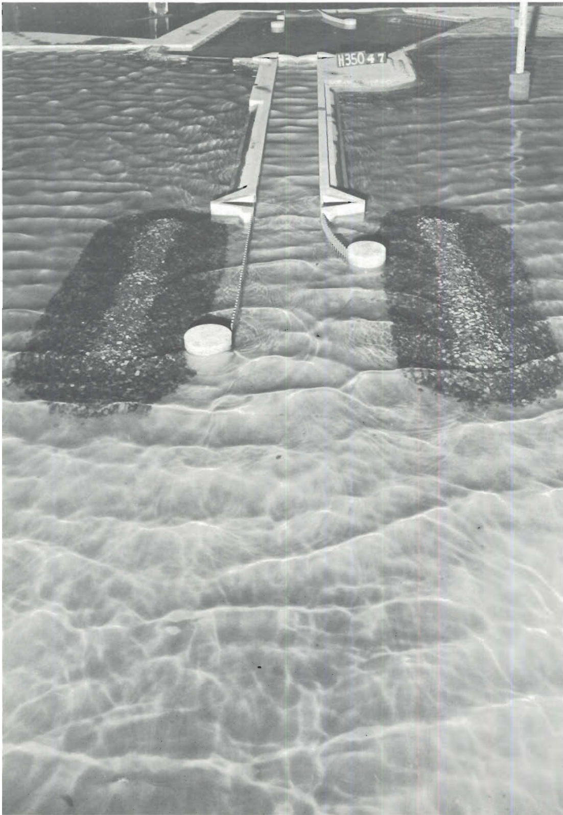
Photo 44. Typical wave patterns at lock entrance for Plan 9; 3-sec, 4-ft waves from NNW; swl = +1 ft msl
