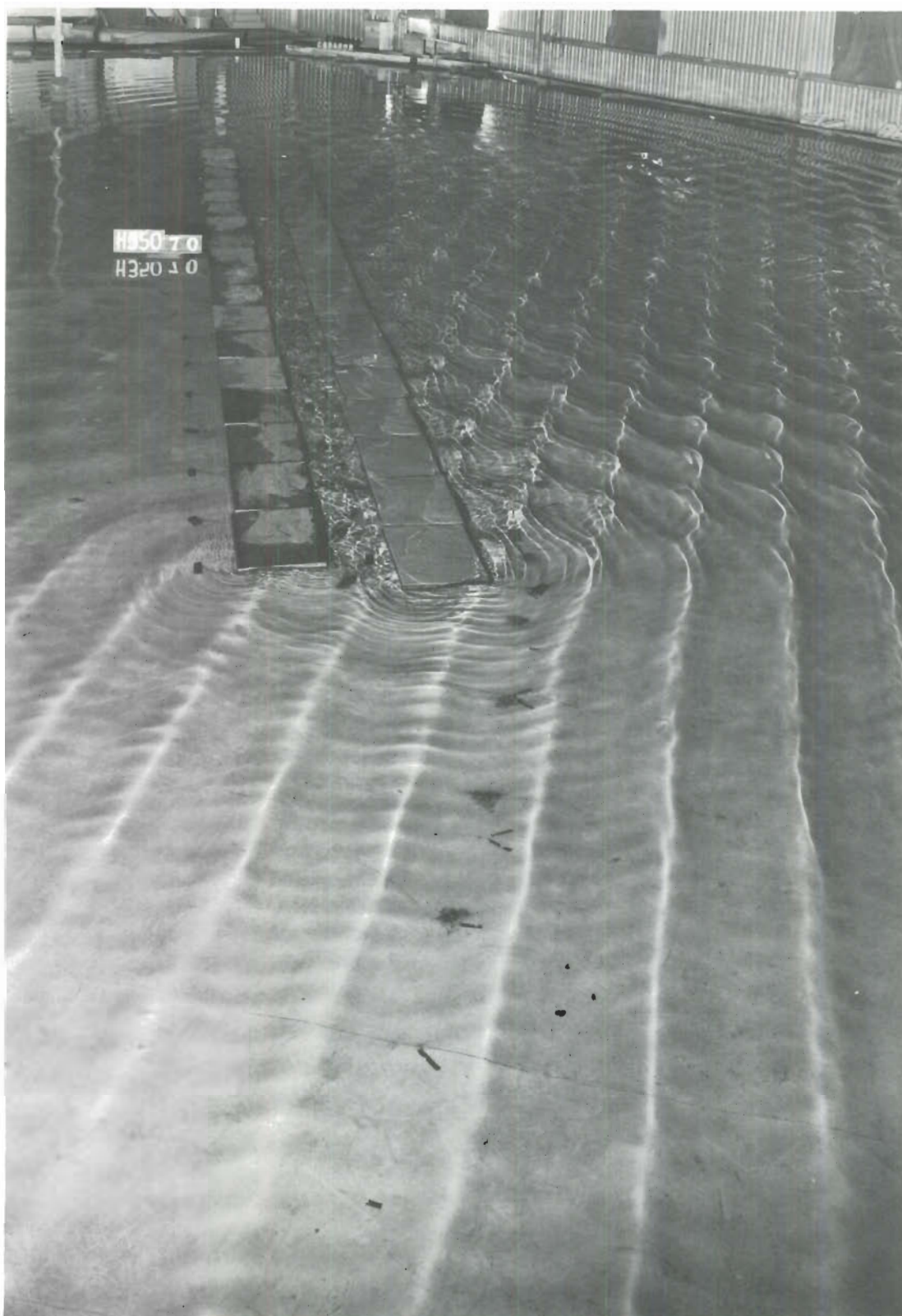
Photo 69. Typical wave patterns at breakwater for Plan 17C; 4-sec, 5-ft waves from N; swl = +1 ft msl
