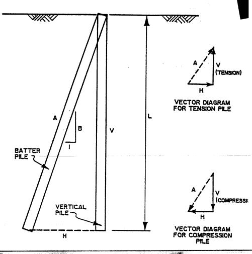
A = ALLOWABLE AXIAL PILE LOAD CAPACITY OF A SINGLE BATTER PILE ESTIMATED AS FOLLOWS:
