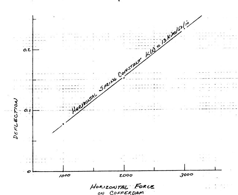
ITERATIONS OF THREE LOADS APPLIED TO COFFERDAM TO DETERMINE SPRING CONSTANT FOR THE CFRAME PROBRAM.
