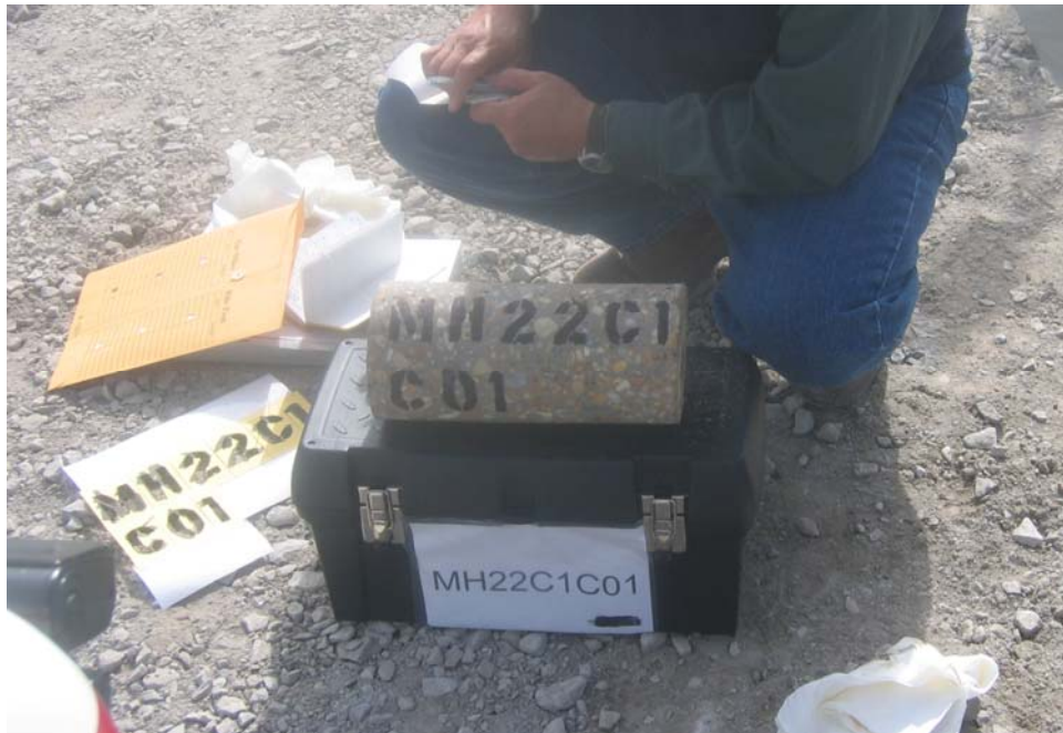
Figure K4-10. Cylindrical core from wall panel H22
