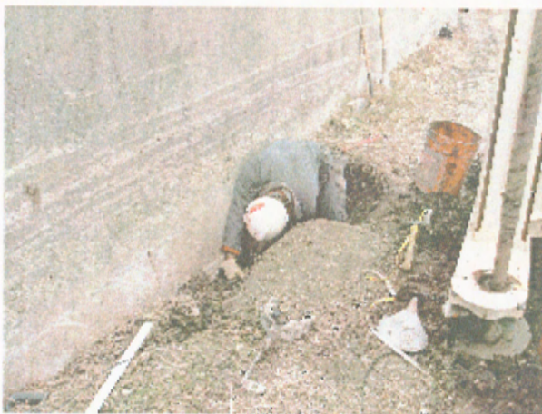
Photo 9 - IHNC 3-lb Impulse hammer impacts to sheet pile on canal side at Station 17+11
