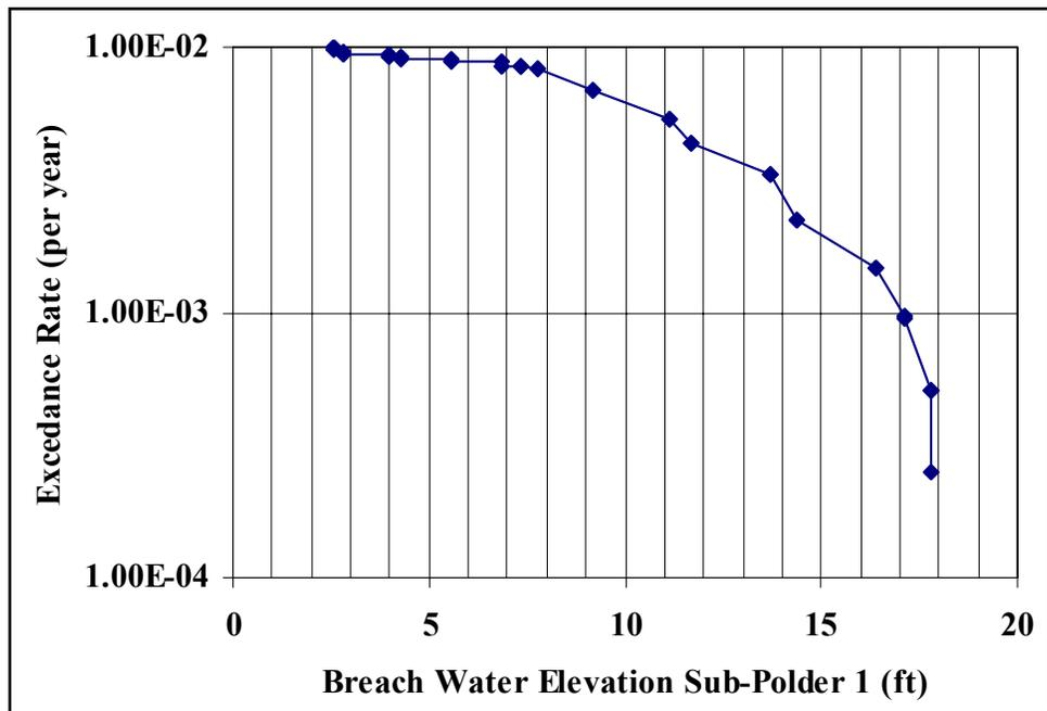
Figure VIII-5. Breach Risk Profile for Sub-Polder 1
