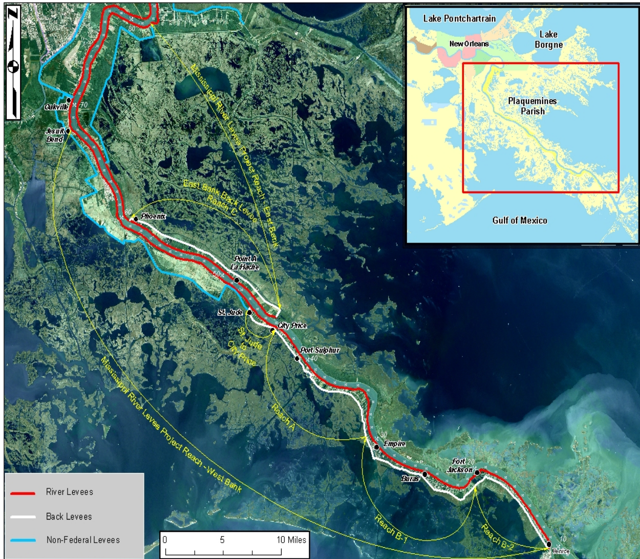
Figure IV-2. Extent of NOV Hurricane Protection in Plaquemines Parish. The NOV consists of five distinct reaches; Reach C, Reach St. Jude to City Price, Reach A, Reach B-1 and Reach B-2.
