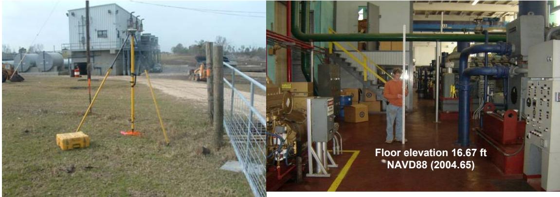
Figure III-25. (Left) Static GPS survey to establish elevation on a benchmark outside a St. Bernard Parish pump station. (Right) Leveling first floor elevation inside Jefferson Parish Pump Station No. 3.
