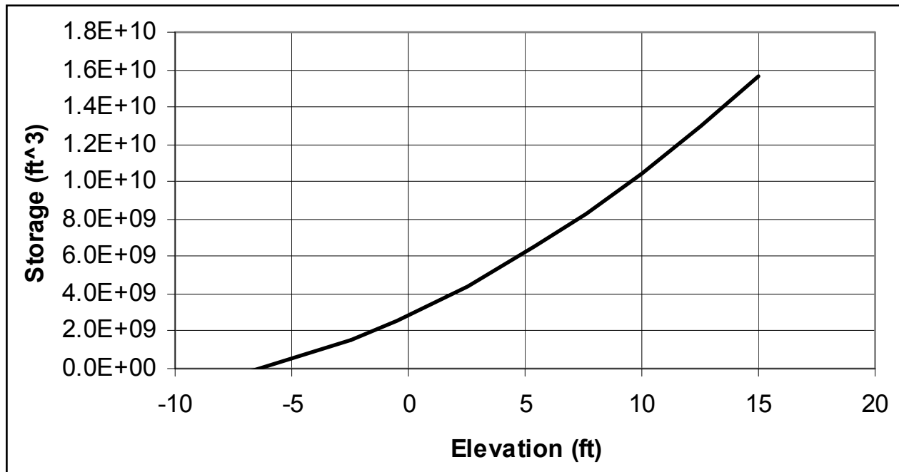
Figure 9-10. Typical Stage-Storage Curve
