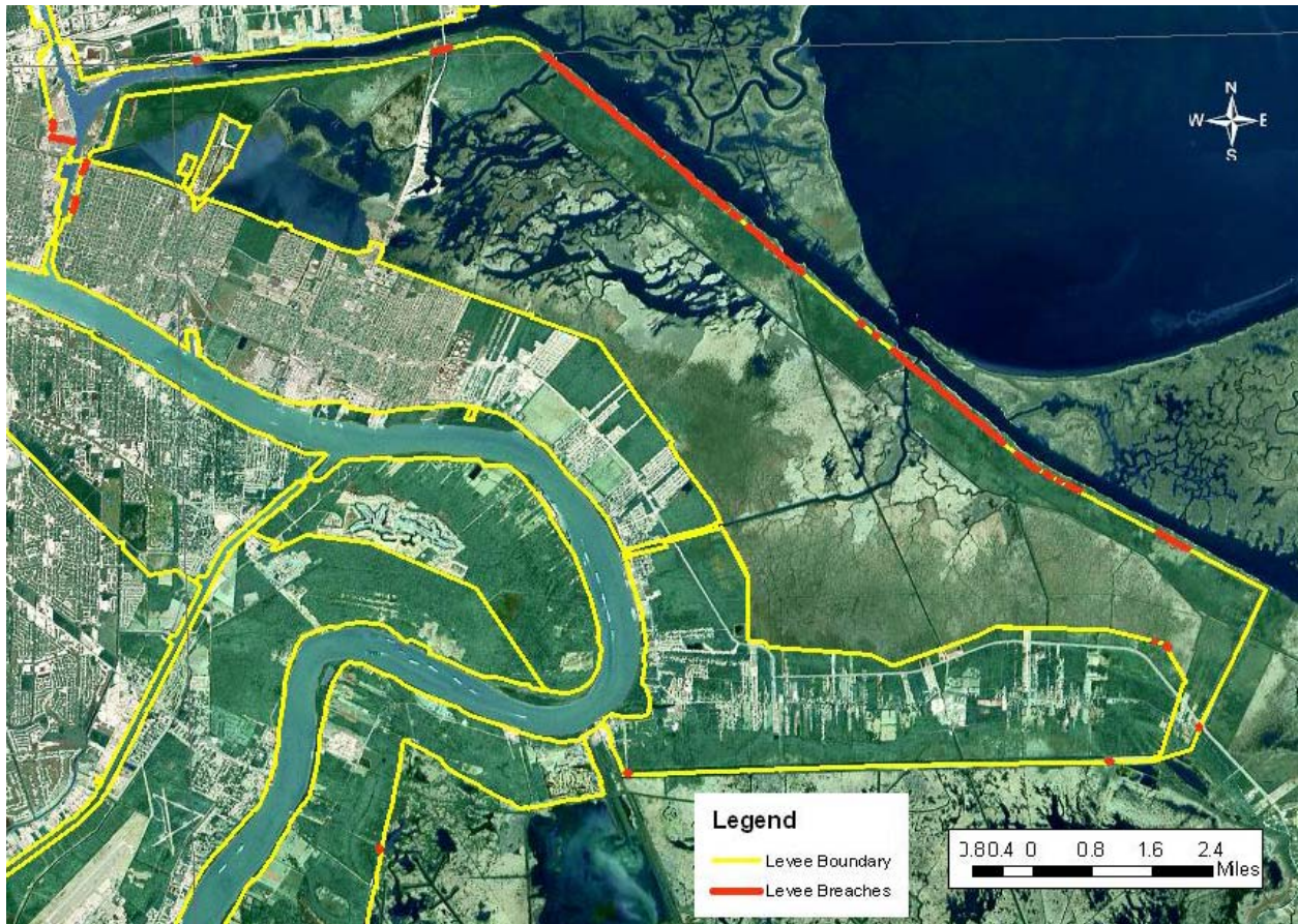
Figure 97. St. Bernard Parish breach locations.
