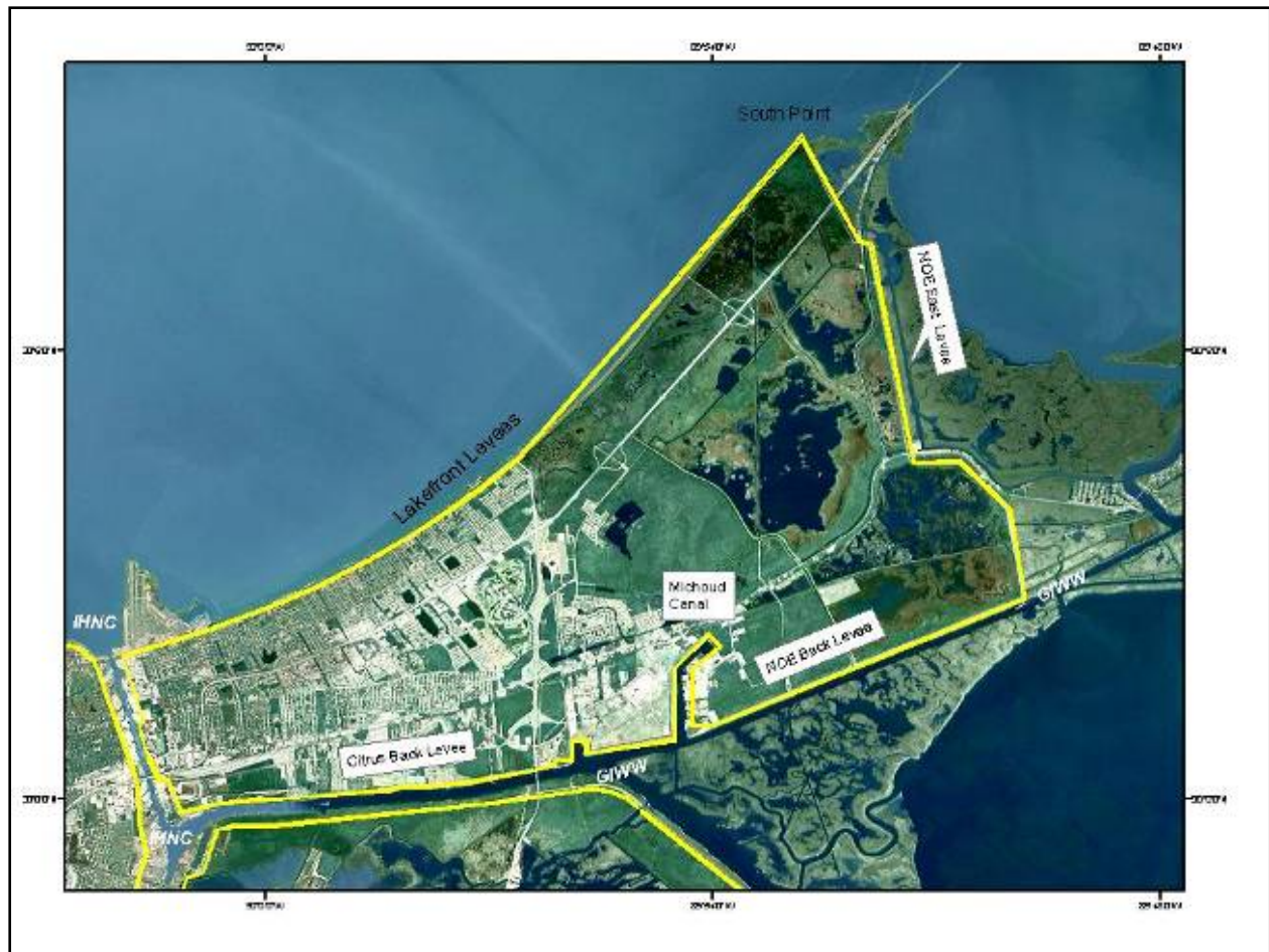
Figure 84. General map of NOE basin. Major levee segments are Lakefront levees, NOE east levee (South Point to GIWW), NOE back levee, Citrus back levee, and IHNC levees.
