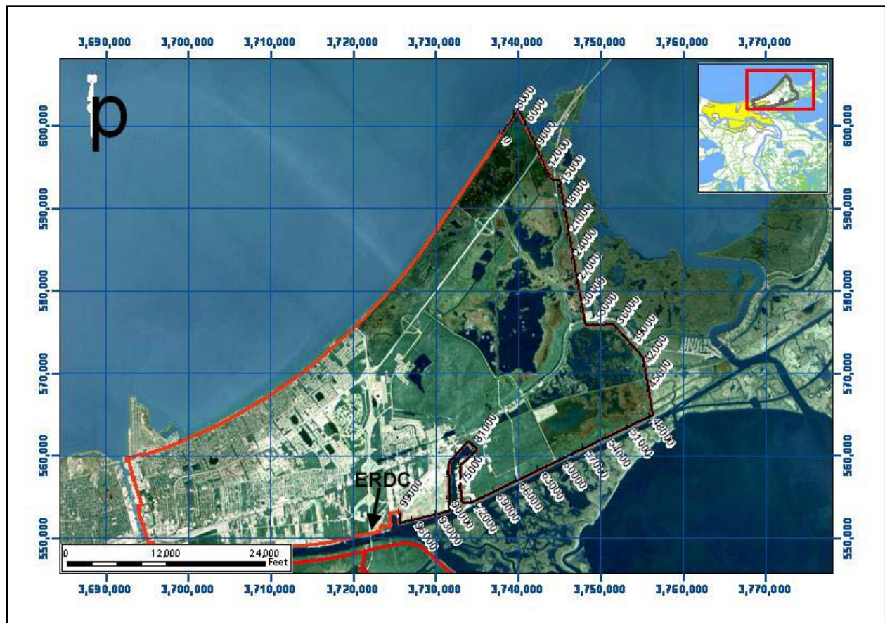
Figure 89. LIDAR stationing used in this report, starting at Lakefront levee and ending at the Michoud Slip along the GIWW.
