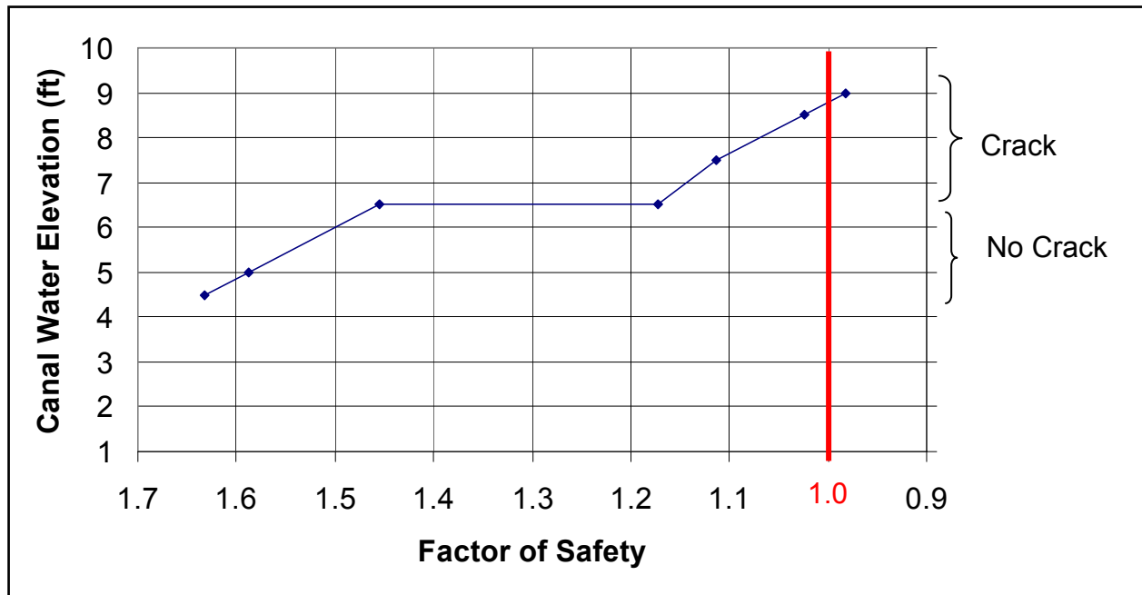
Figure 29. Factor of safety versus canal water elevation computed in the soil-structure interaction analysis of Station 10+00 on the 17th Street Canal east side breach.
