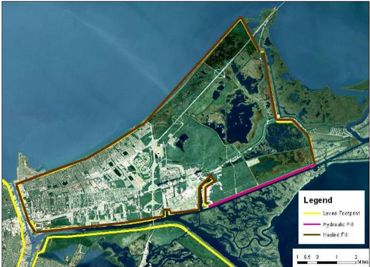
Figure 86. NOE Levee construction materials.
