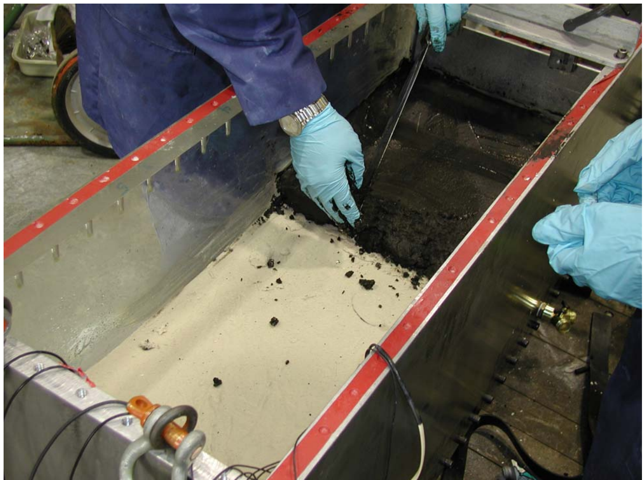
Figure 5.80. View of placement of swampy/marsh layer
