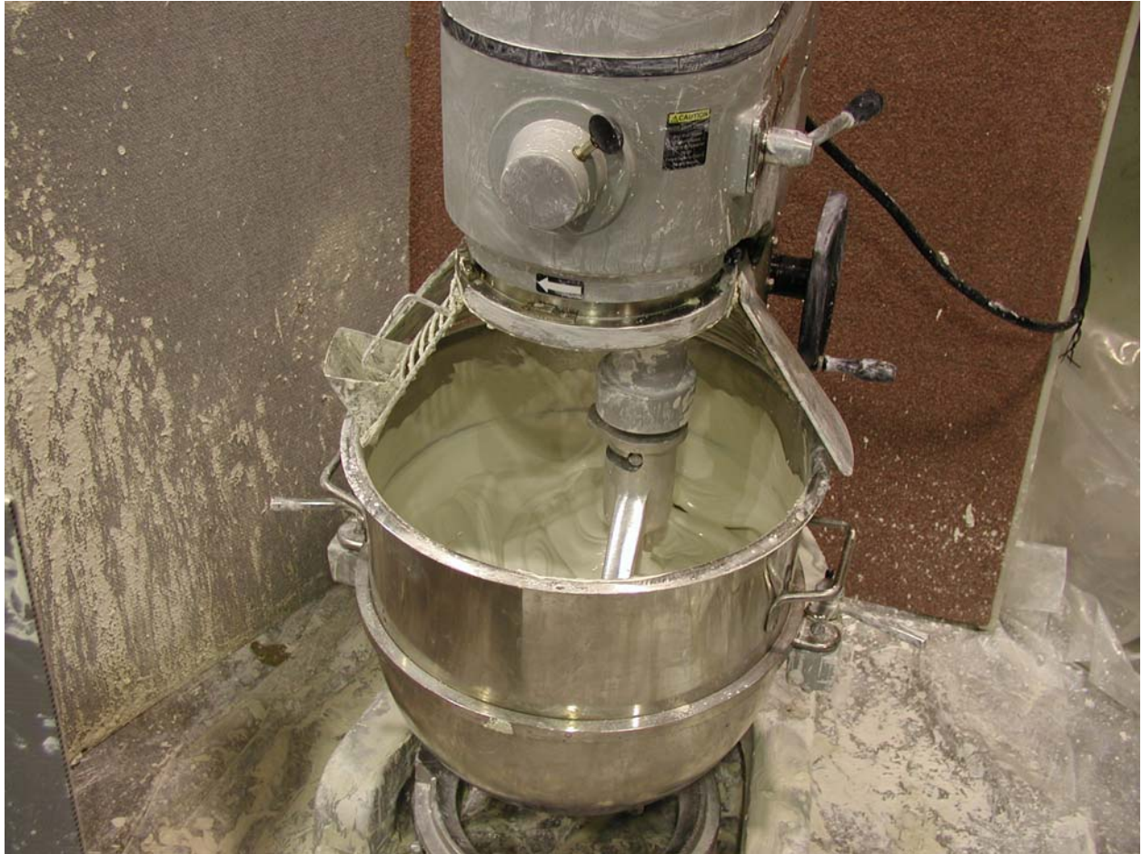
Figure 5.42. View of the clay mixing process
