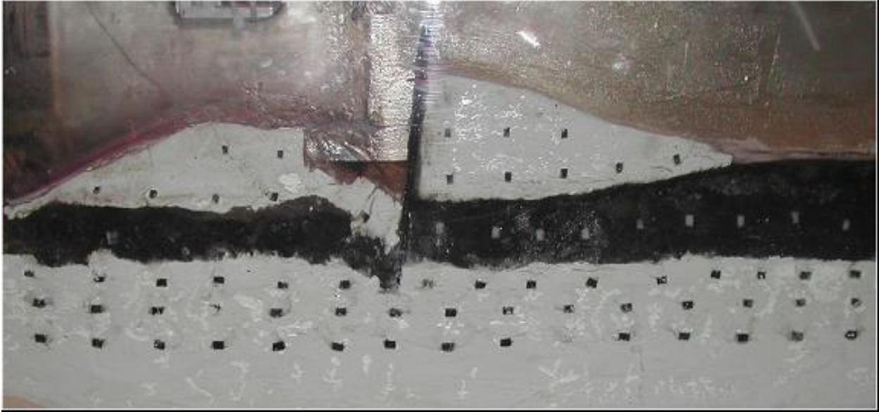
Figure 5.31. Final state of 17th Street Model 1 showing lateral translation on sliding surface starting at the toe of the wall and progressing landwards.
