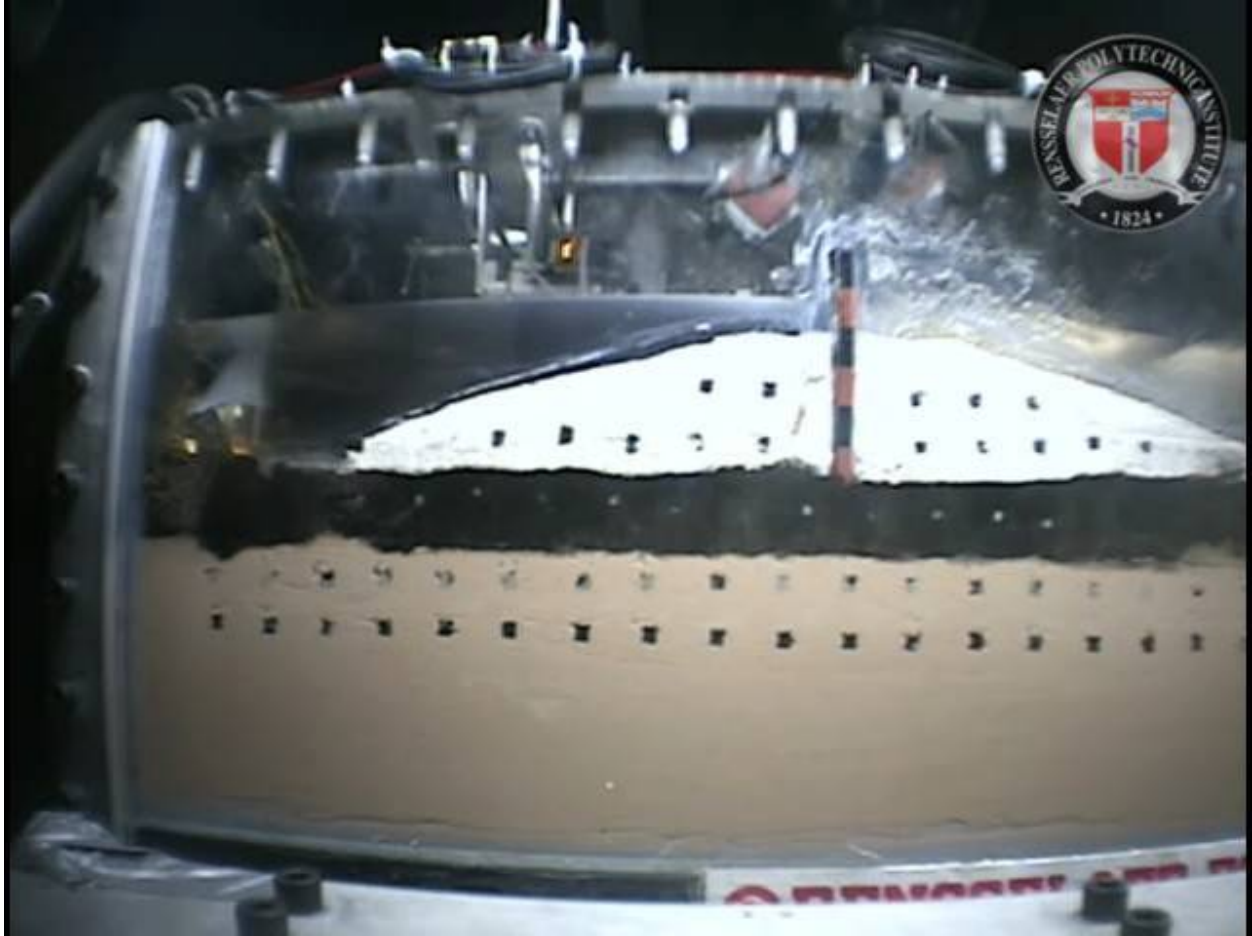
Figure 5.102c. View of RPI Orleans south model at Hurricane Katrina flood level, held here for long period
