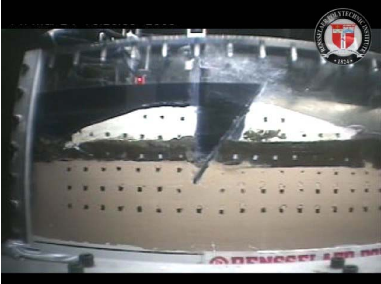
Figure 5.77g. RPI London south model at end of failure
