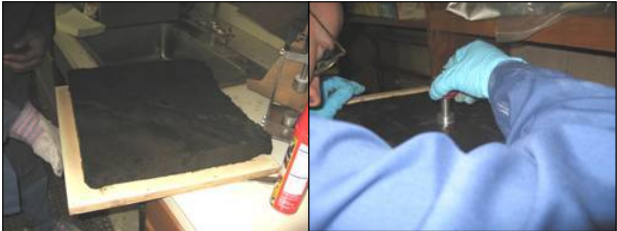
Figure 5.79. Swampy/marsh layer and taking vane shear measurements
