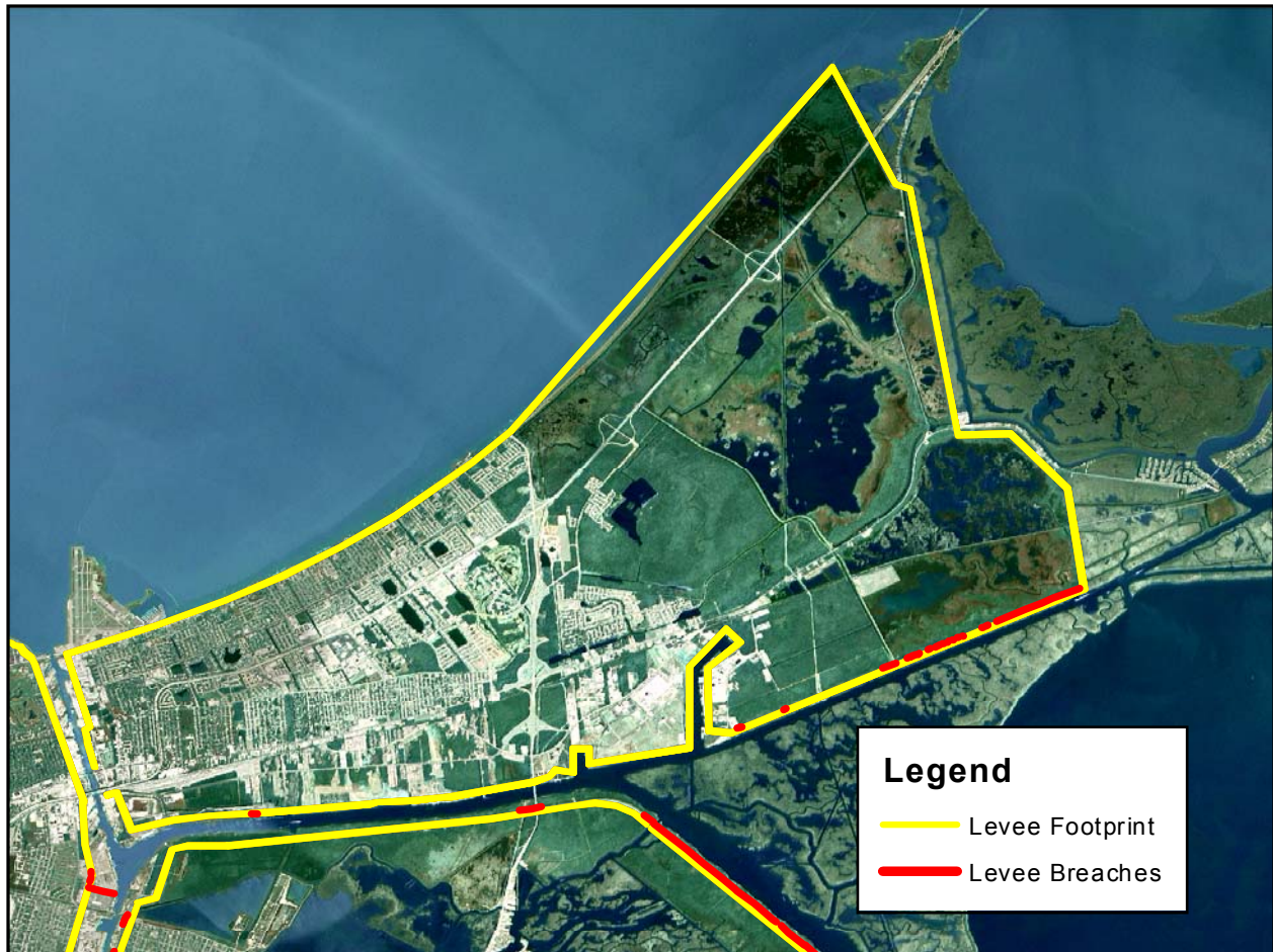
Figure 19b. Distribution of levee breaching, New Orleans East and northern St. Bernard.
