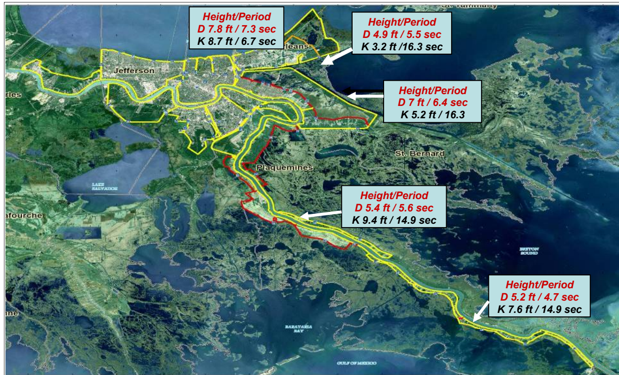
Figure 15. General comparison of wave height and period assumed in HPS design (D) and estimated from Katrina (K). See Volume IV for more detailed information.
