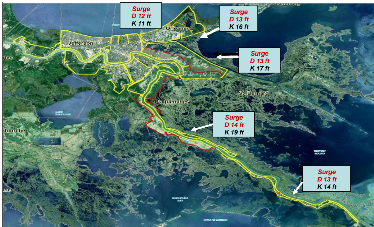
Figure 14. Comparison of general surge levels assumed in the SPH design (D) and estimated from Katrina (K). See Volume IV for more detailed information.
