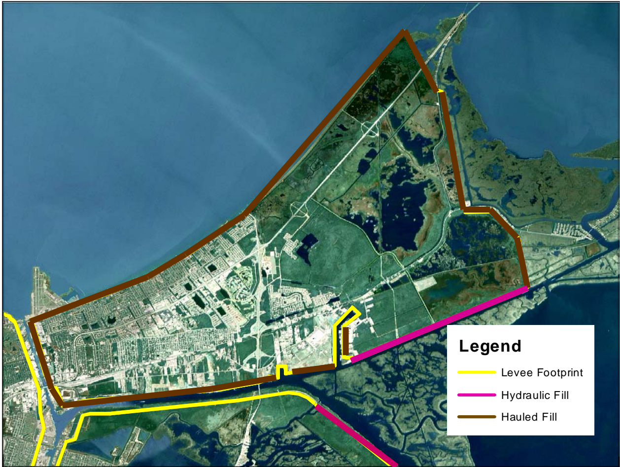
Figure 19a. Character of levee materials, New Orleans East and northern St. Bernard. This slide is incomplete for St. Bernard and shows only the hydraulic fill section along the MRGO.
