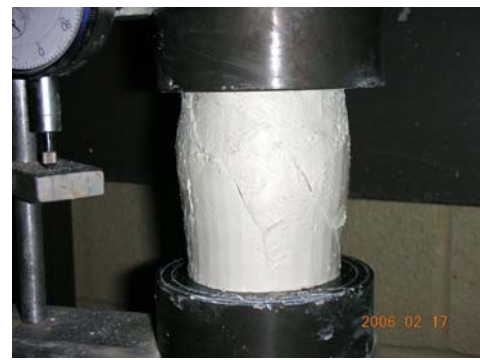
Shear Strength Estimation of Clay Layer @17th street
