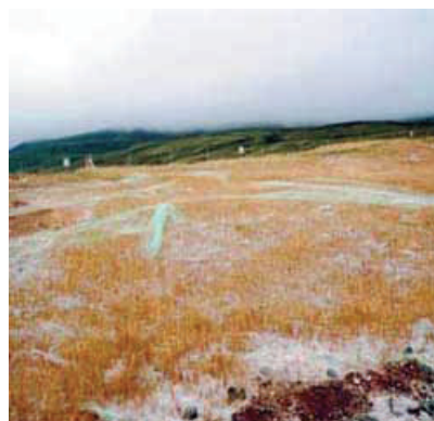
Figure 90: Damage to an excelsior blanket product when used in severe wind areas. The plastic backing separated from the wood fiber and created a non-degradable mess capable of entrapping small wildlife.
