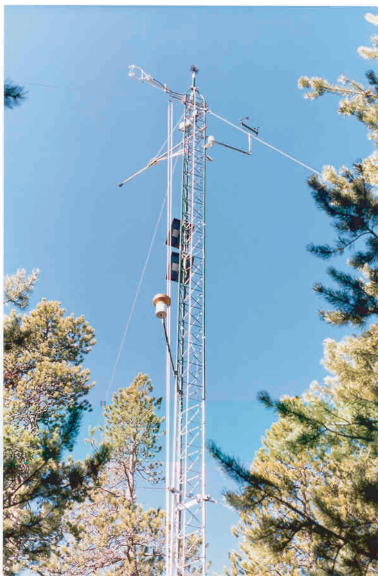
Figure 9. Eddy-correlation evapotranspiration tower at forest site.
