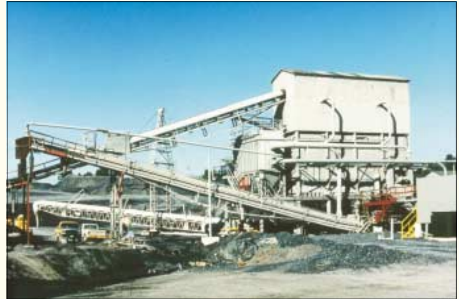
Figure 13. Noisy equipment can be located away from populated areas and can be enclosed in sound-deadening structures. (Photograph courtesy Luck Stone.)
