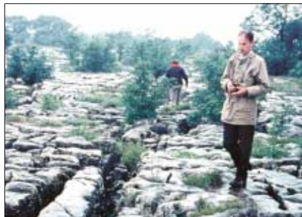
Figure 6-b (far right, top and bottom). Removal of overburden has exposed the furrowed and pitted surface of carbonate rock. (Photograph courtesy of Keith Bennett, Williams Earth Sciences, Inc.)
