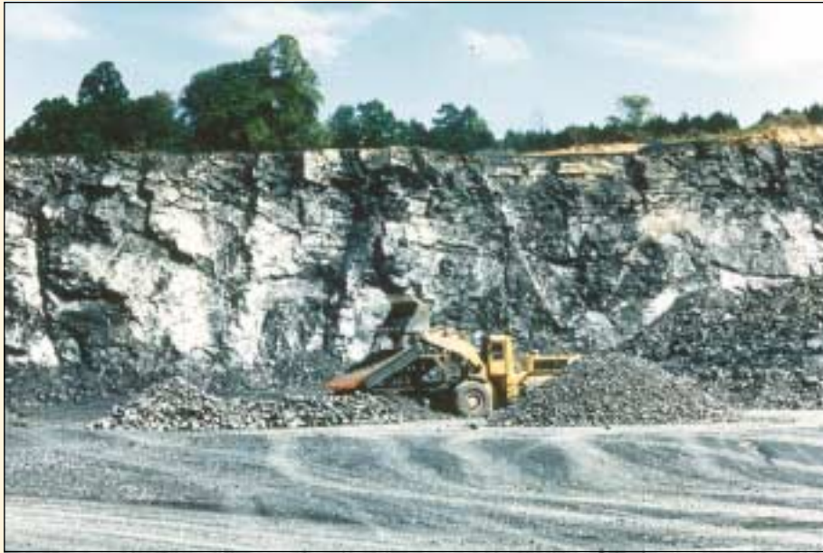
Figure 8. Working face of crushed stone operation showing rubble created by blasting. (Photograph courtesy Luck Stone.)
