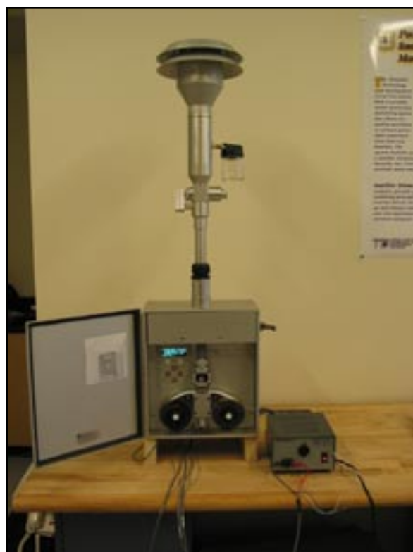
Figure 3—The E-BAM monitor with its environmental door open. The instrument collects particulate on a filter tape that automatically advances when the tape is full.
