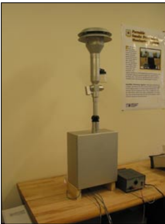
Figure 2—MetOne Instruments' E-BAM monitor is a portable real-time beta-attenuation PM_{2.5} and PM_{10} particulate monitor.
