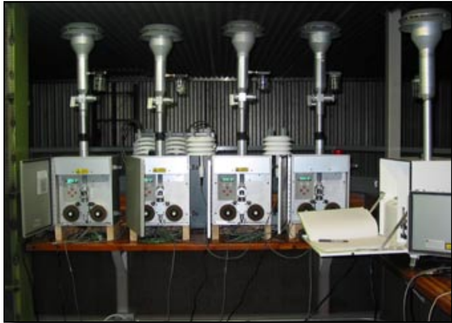
Figure 6—The E-BAM monitor was tested in the Rocky Mountain Fire Sciences Laboratory's smoke chamber.
