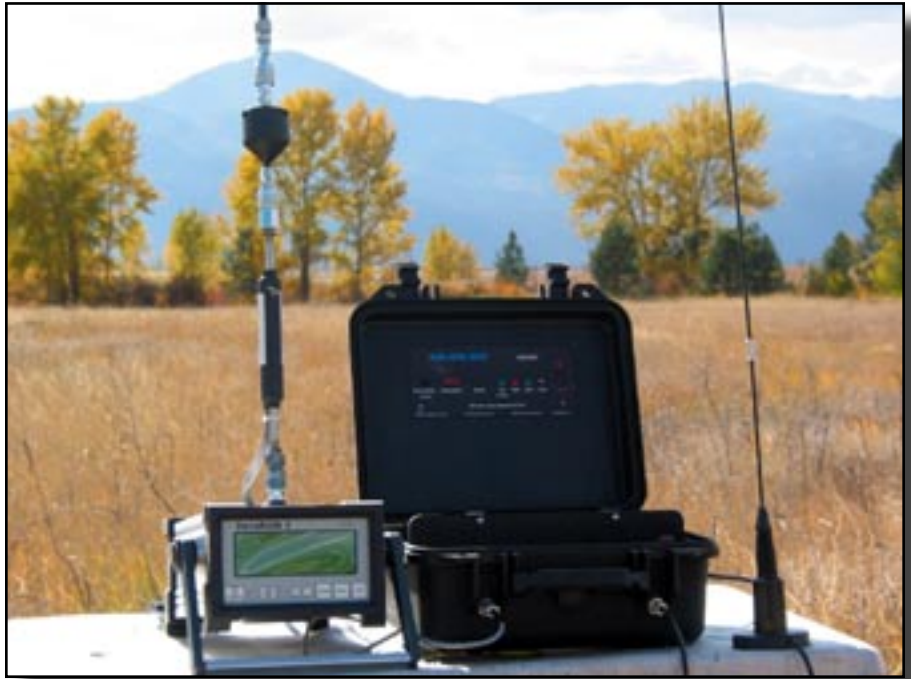
Figure 5—The Thermo-Electron MIE DataRAM4 (shown with satellite telemetry system) is a dual-wavelength, light-scattering device that estimates particulate concentrations.
