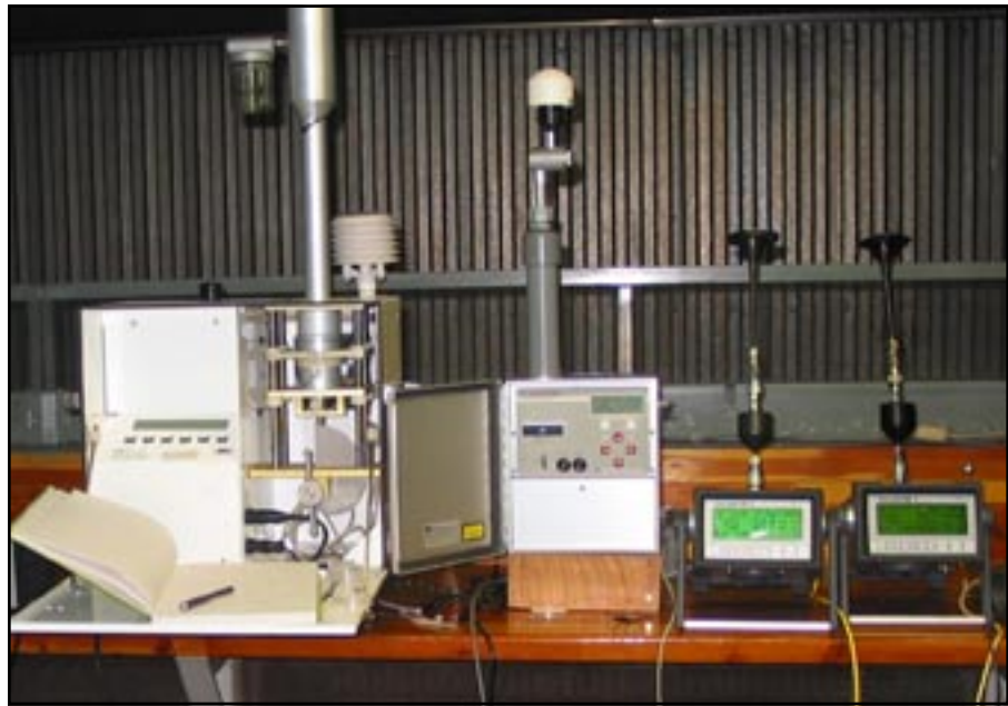
Figure 7—The BGI PQ-200 Federal Reference Method sampler (left) with MetOne Instruments' E-Sampler (middle) and the two DataRAM4 monitors (right).
