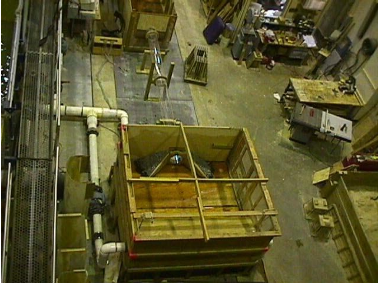
Figure 3. Test facility set up for Dale Boulevard culvert.
