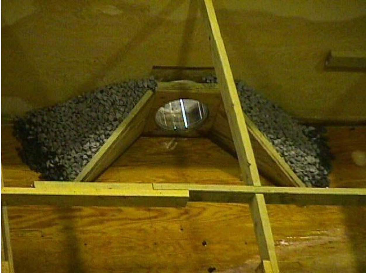
Figure 4. Inlet of test facility set up for Dale Boulevard culvert.
