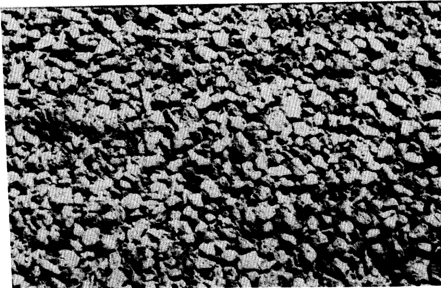
Photo No. 5. Cement-Treated Permeable Base
