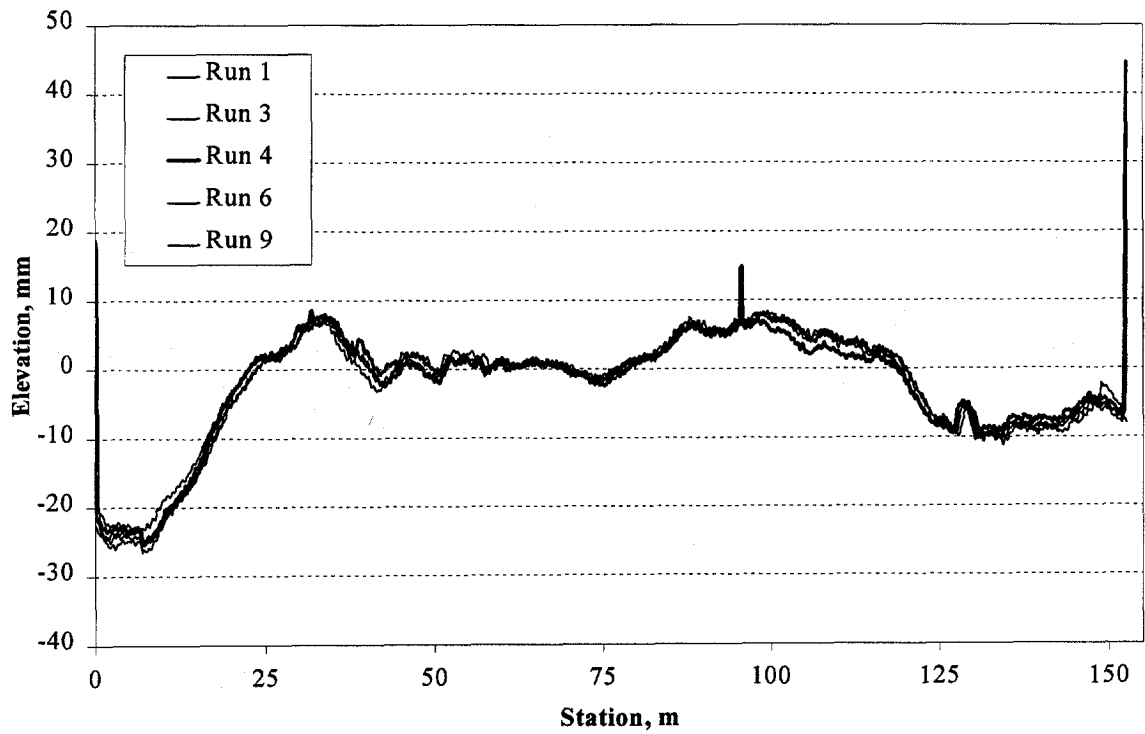
Figure 38. Unnoted saturation spike in right wheelpath profile from Ontario.
