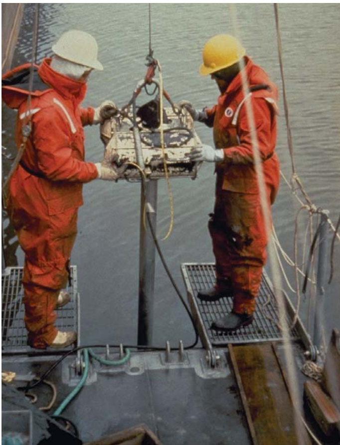
Sediment sampling aboard EPA research vessel, "Mud Puppy" in Indiana Harbor Canal
