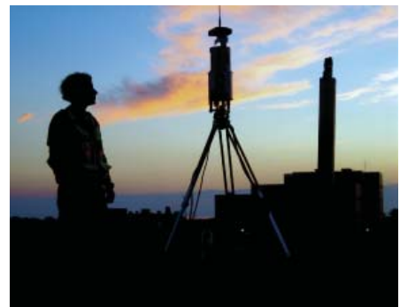
USGS Mendenhall Postdoctoral Research Fellow Brian Collins collects terrestrial lidar data at the Kashiwazaki municipal-incinerator landslide site.
