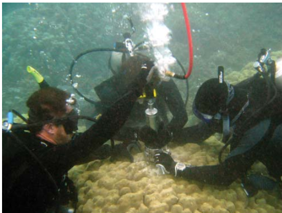
USGS scientists drill into a coral head to obtain a core for study of the impacts of sediment in runoff from Moloka‘i.
