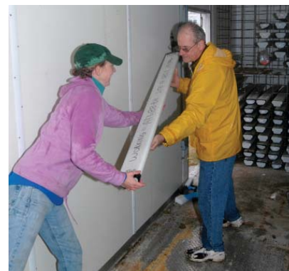
Elizabeth Pendleton (left) and Greg Miller remove "D tubes" (named for the shape of their cross section) containing split core halves from the old refrigerated vans. Photograph by Dann Blackwood .
