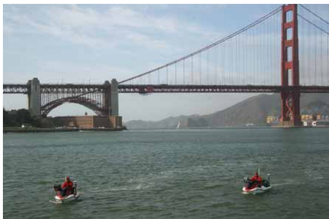
Patrick Barnard and Jeff Hansen using CPSes to obtain bathymetric data. The Golden Gate Bridge is in the background. Photograph by Tom Reiss , October 26, 2007.
