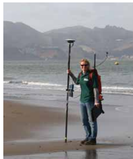
Li Erikson carrying backpack and antenna for beach-profile measurements. Photograph by Tom Reiss , October 26, 2007.
