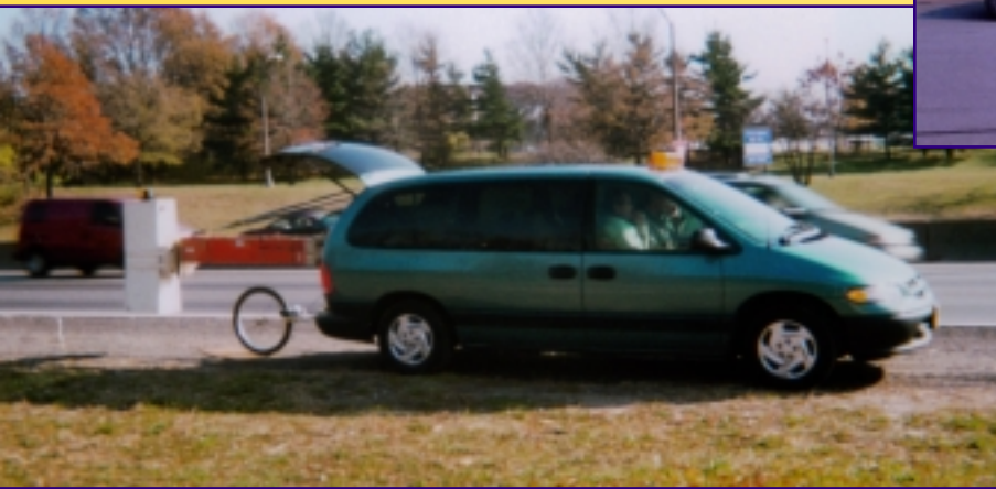
FIGURE 6: Portable GPR Equipment Mounted on Rented Vehicle
