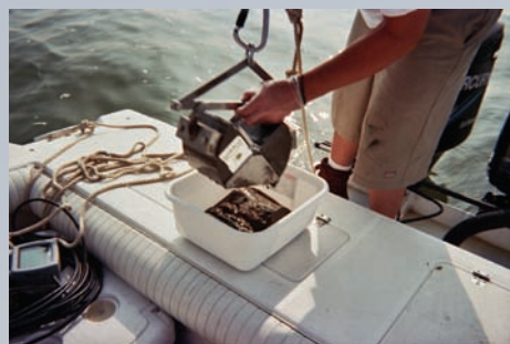
Picture 1. Petite Ponar Grab sampler is used to collect bed sediment at Maumee River and Offshore sites.
