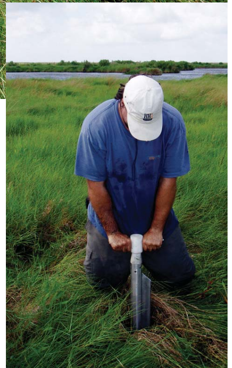
Kyle Kelso plunges a Russian peat corer into the ground at Sabine National Wildlife Refuge to recover a core sample. Core data are being used to determine whether specific wetland areas have eroded or subsided relative to sea level.
