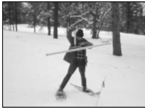
Measuring water content of the snow pack on Willow Creek, White Mountain Watersheds, Arizona.
