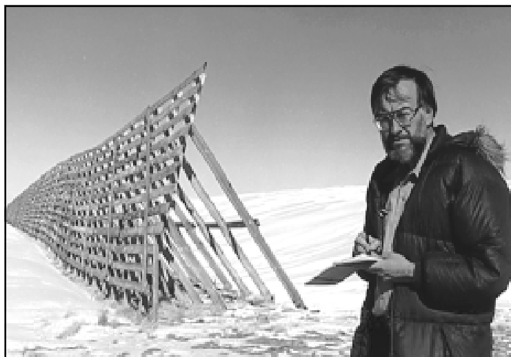
Ron Tabler, Laramie, records data on snow accumulation behind one of the snow fences protecting Interstate 80 west of Laramie, WY (1982). Engineered snow fences can trap large amounts of blowing snow in long drifts higher than the fences (which may be 12 feet tall), greatly reducing plowing costs and highway closures, improving visibility along the highway, and providing water for livestock and wildlife during snowmelt.
