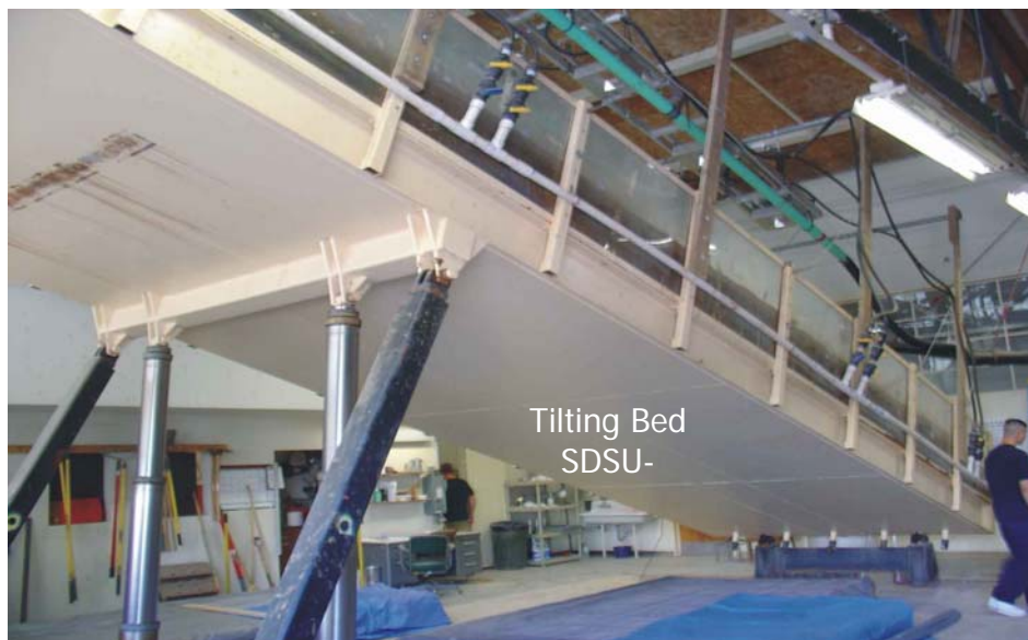
Figure 2-5. Tilting Test Bed (underside view)
