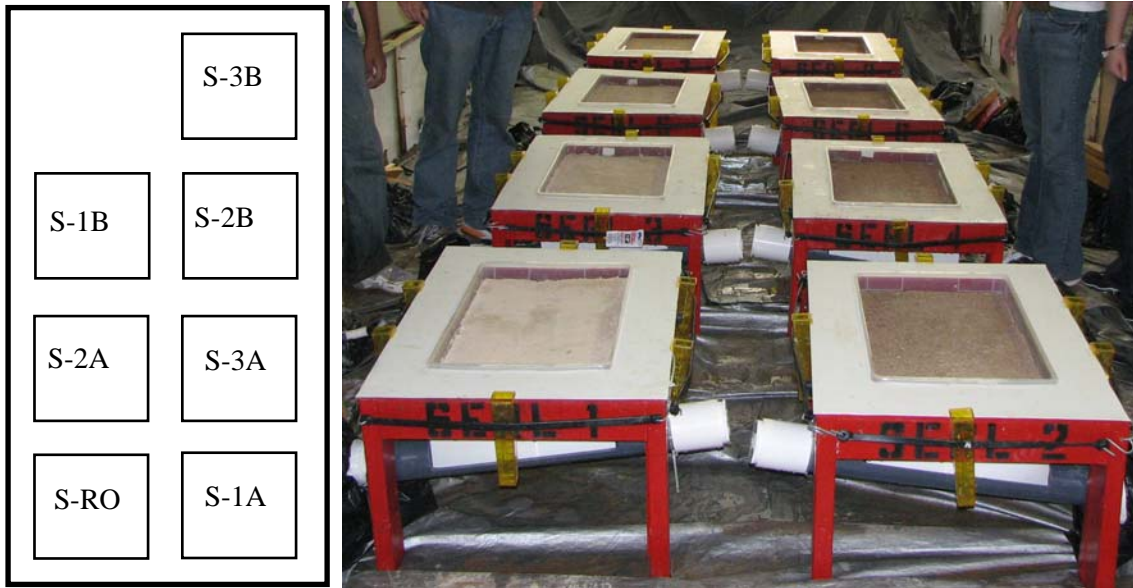
Figure 2-11. Plan view of tilting soil bed with approximate location of soil test boxes; drawing not to scale, where S is soil type; 1, 2, 3 are products; A and B are product application scenarios.
