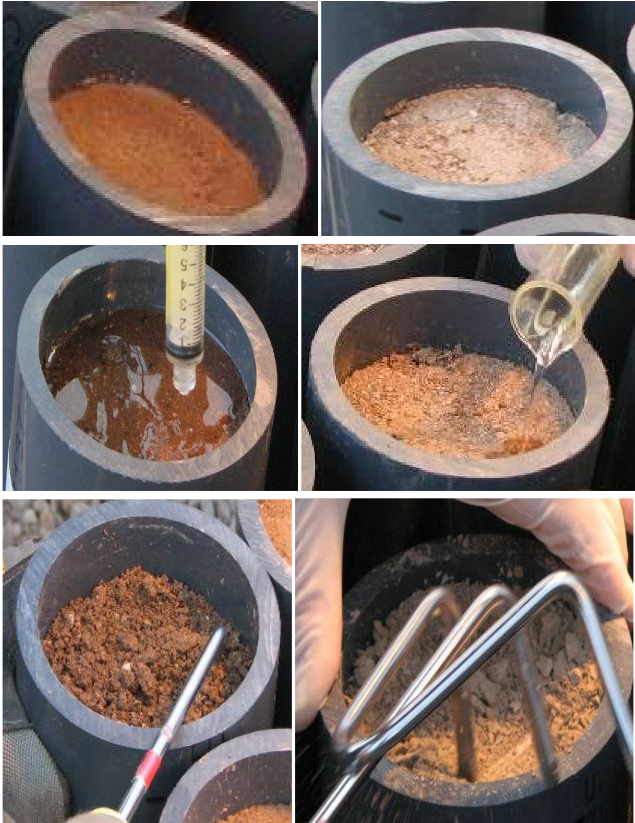
Figure 2-13. Typical AZ (left) and NV (right) soil columns before and after product application and raking
