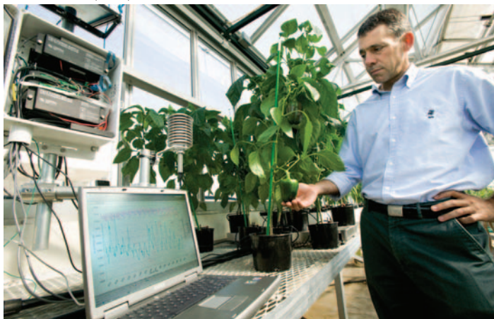
Ron Seligman observes a data acquisition and control system used in a greenhouse study of nutrient and water uptake by pepper plants.
