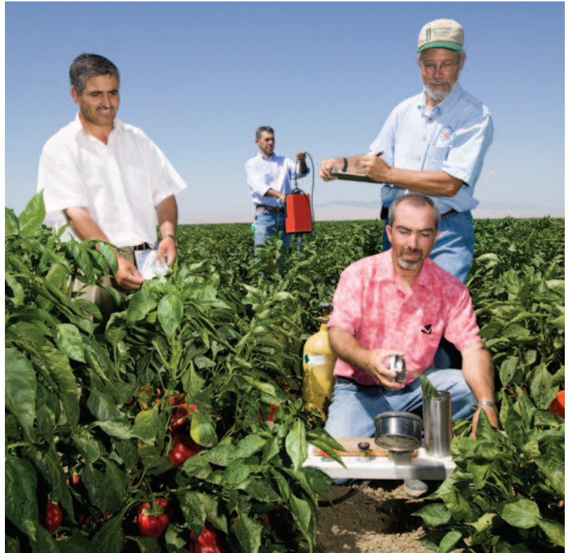
Naem Mazahrih (left), Nedal Katbeh-Bader (kneeling) and ARS research leader Tom Trout (holding the clipboard) use a pressure chamber to check pepper plants’ water status while Ron Seligman (in the background) checks soil water content with a neutron probe.
