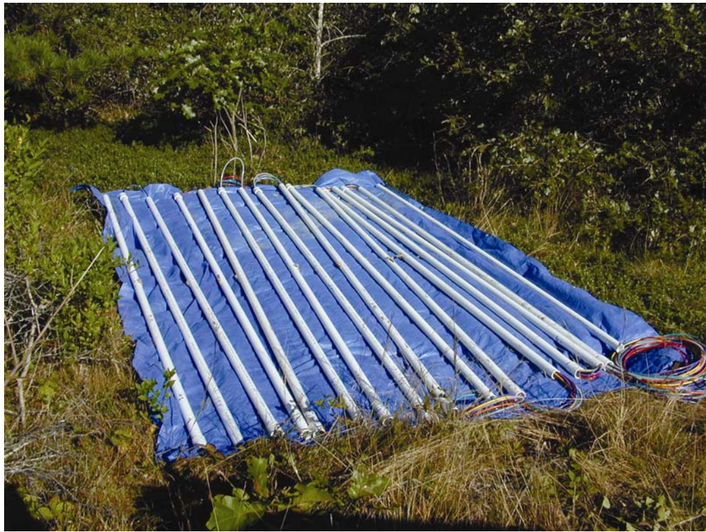
Figure 20. Multilevel sampler before installation at Prince Valley Road. Each pipe segment is nominally 10 feet long. Internal tubing emerges through the PVC segments at their midsections.
