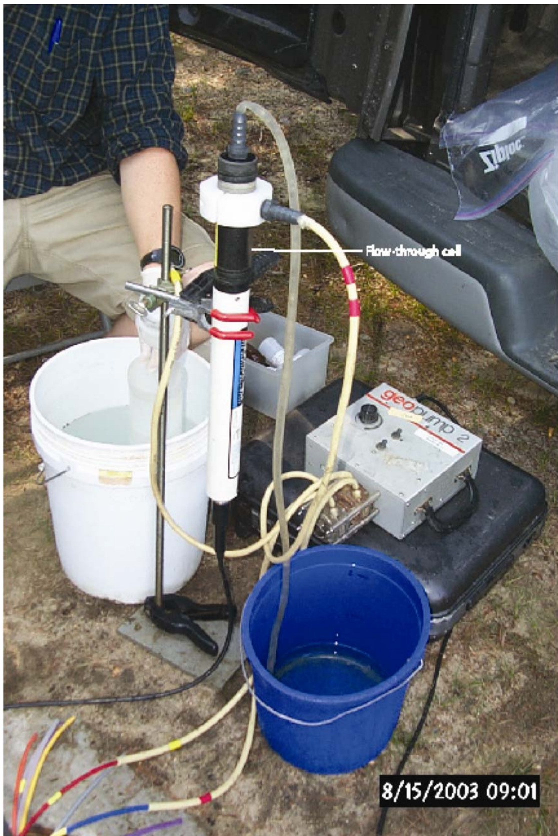
Figure 24. Flow-through cell for field measurements of water quality.
