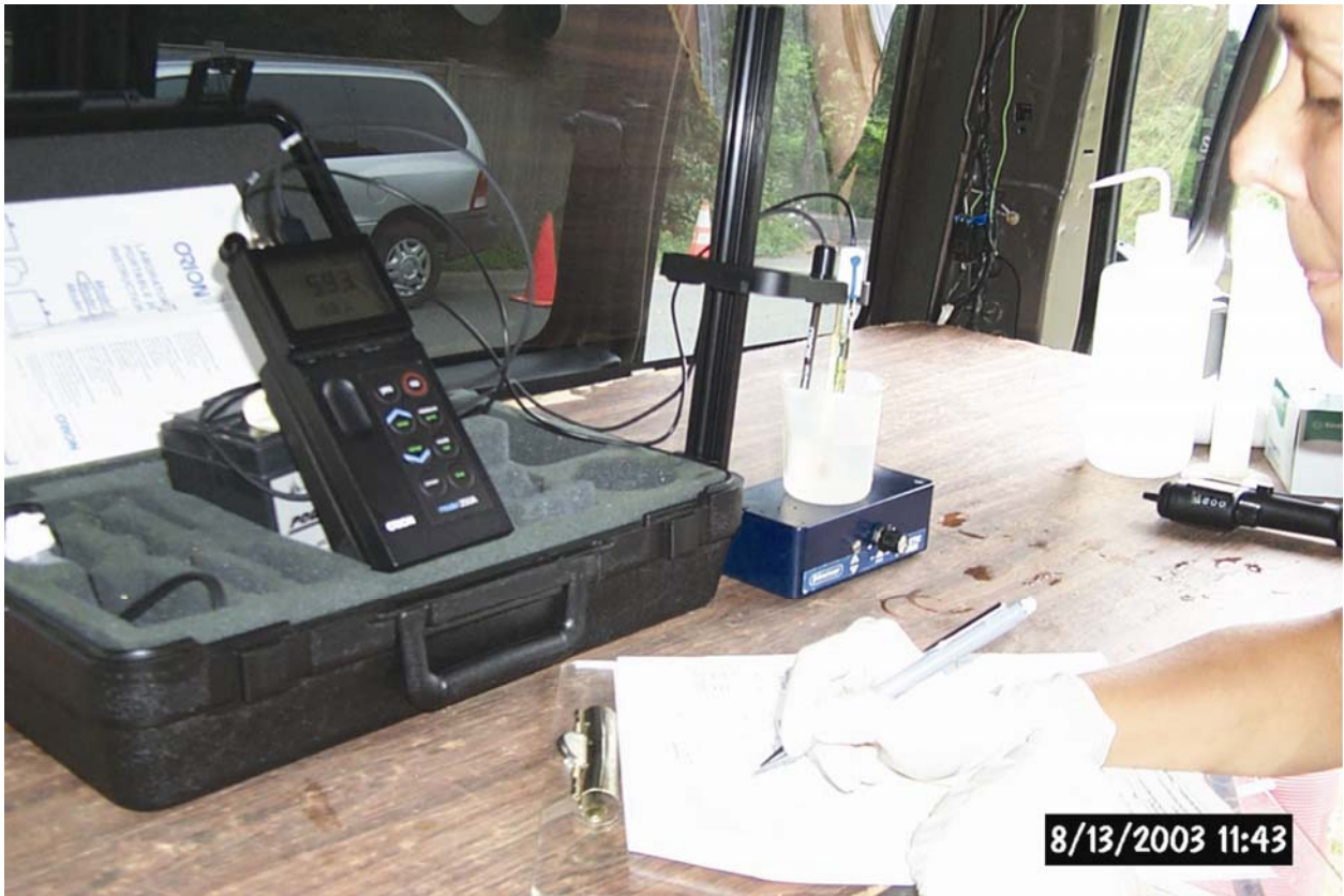
Figure 26. pH meter for alkalinity measurements.
