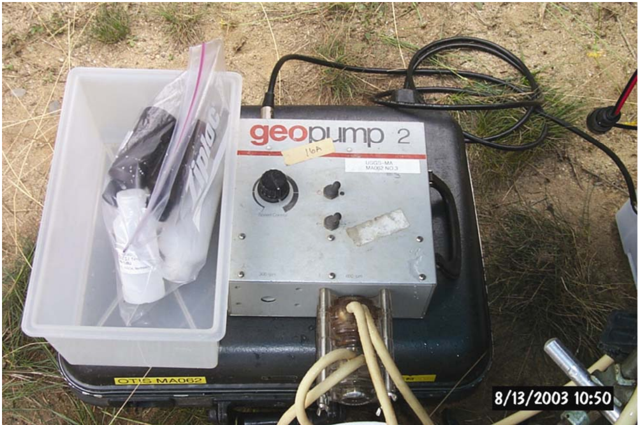
Figure 28. Geopump set up for pumping multilevel sampler ports.
