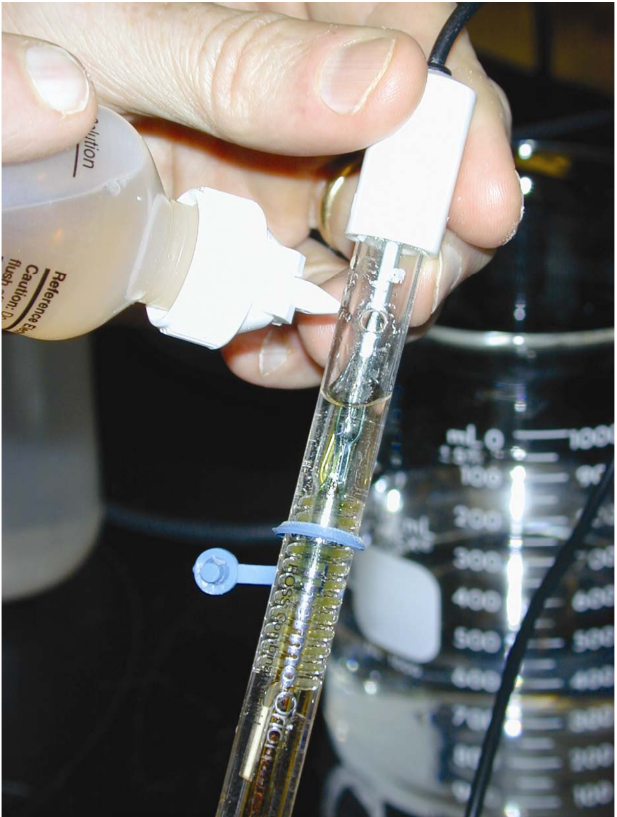
Figure 25. Filling the Ross pH probe with KCl filling solution. The level of the filling solution should be above the level of the surface of the sample during measurement.
