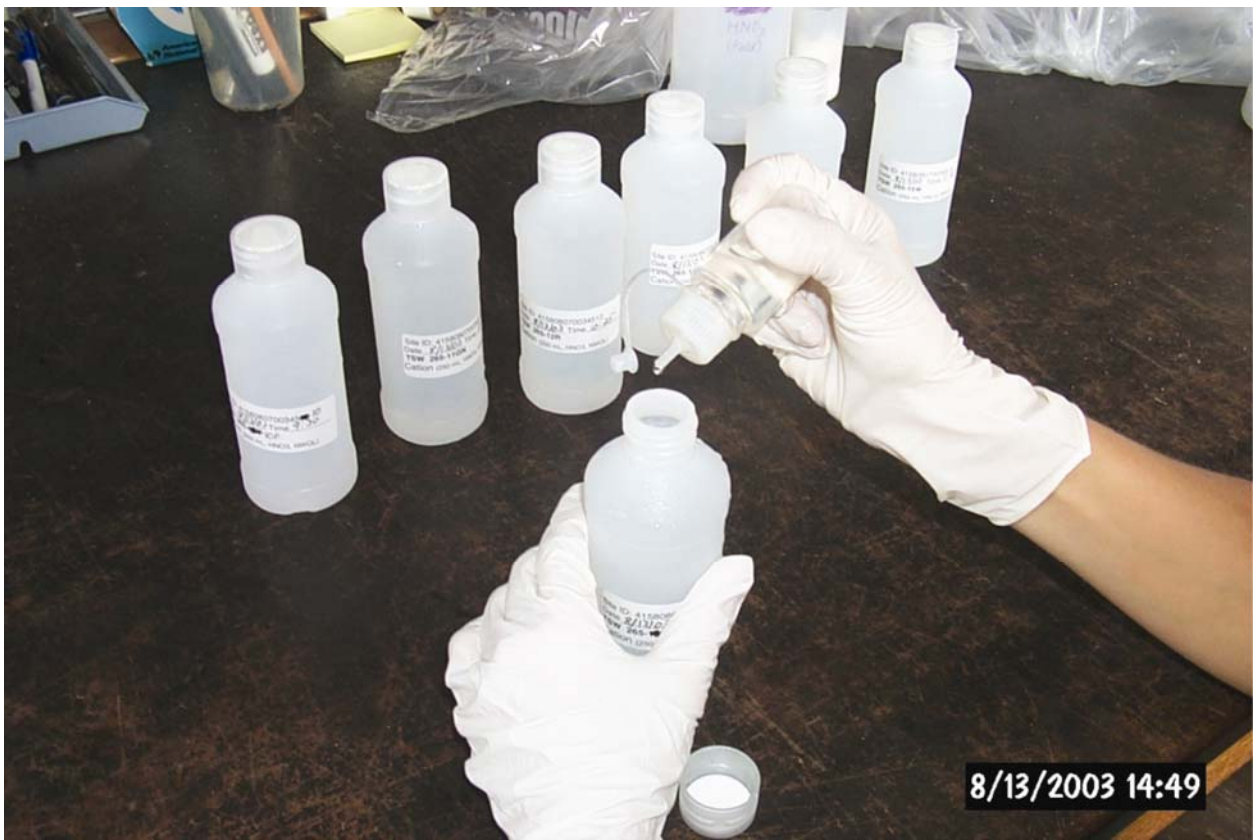
Figure 29. Preservation of samples by using concentrated acid from a Teflon dropping bottle.
