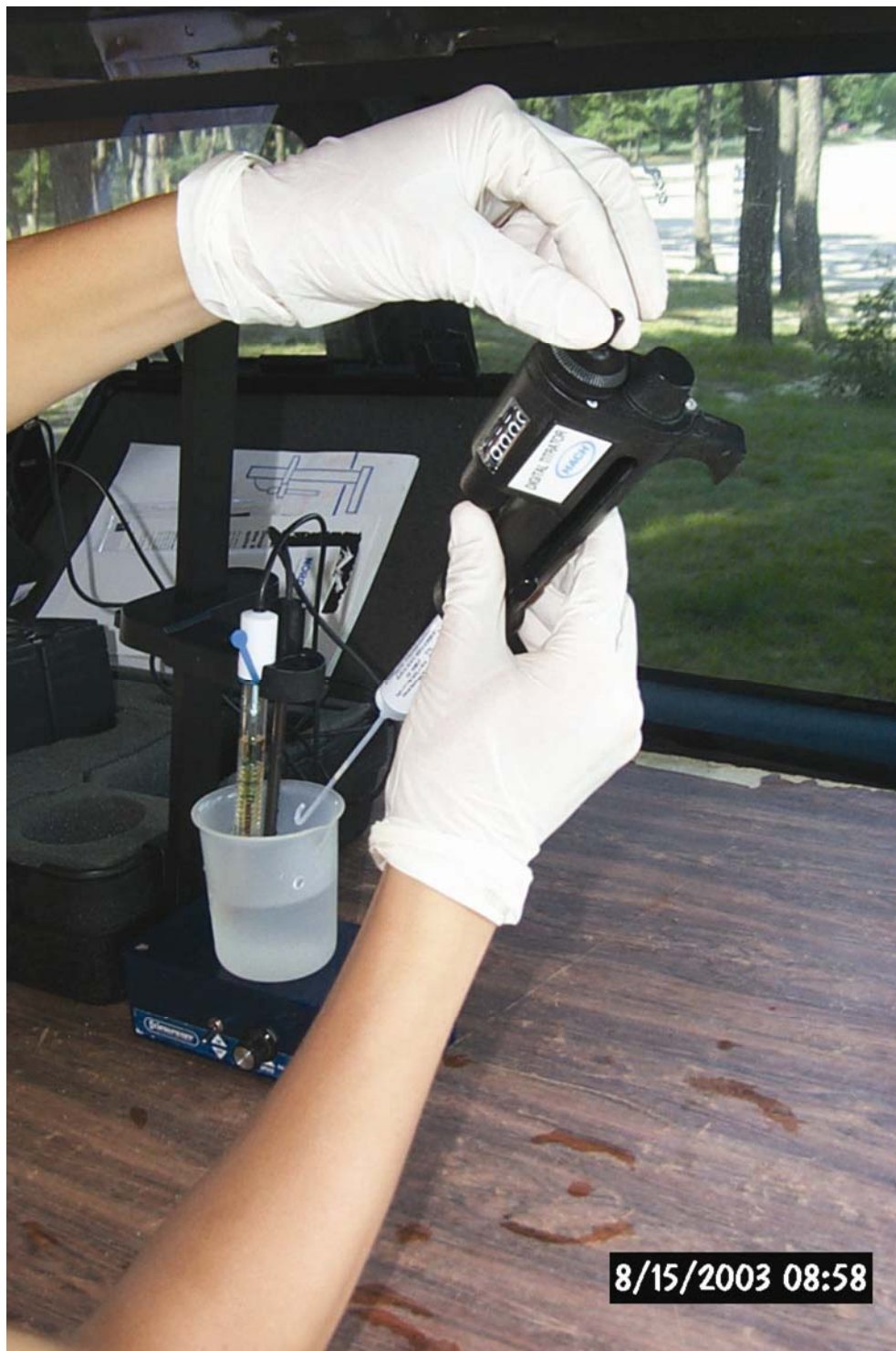
Figure 27. Addition of acid during titration.
