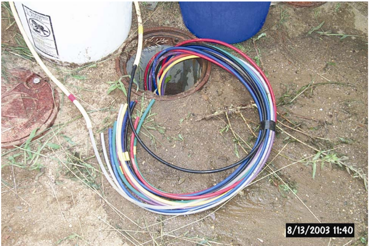
Figure 22. Finished flush-mount multilevel sampler well. Repeat colors are marked with yellow tape.
