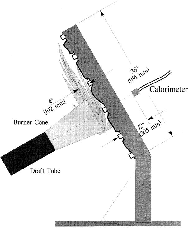
Figure 6 - . Position of Backface Calorimeters Relative to Test Specimen Frame
