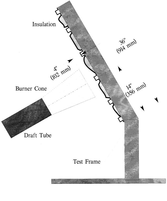
Figure 2 – Burnthrough Test Apparatus
