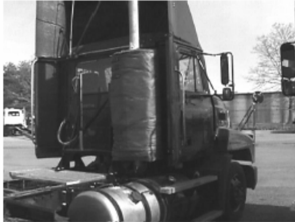
Figure 2-5, Example of an SCR/DPF System Installed on a Heavy-Duty Diesel Truck
