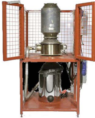
Figure 2-1, DPF Being Regenerated Using External Heating/Cleaning Equipment
