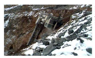
Accident No. 1: A drill toppled over a highwall, crushing the driller, when the support jack near the edge of the highwall sank into soft, unconsolidated material as the tower was being raised.
