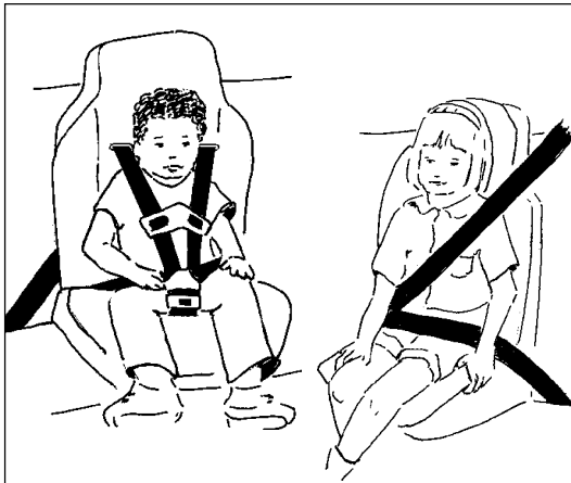
B Child Seat/Booster: This seat (left) has a 5-point harness. If you remove the harness it becomes a belt-positioning booster (right) to use with a lap/shoulder belt for a larger child.
