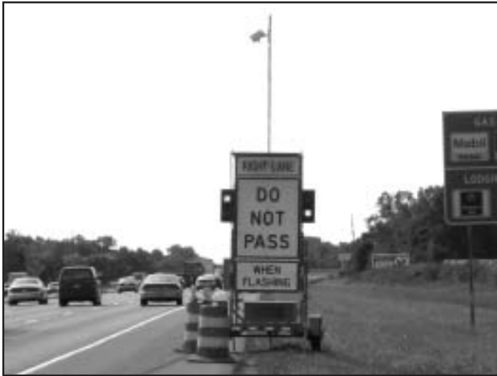
Figure 2 – Activated “Do Not Pass” Sign at the I-94 Dynamic Lane Merge Site
