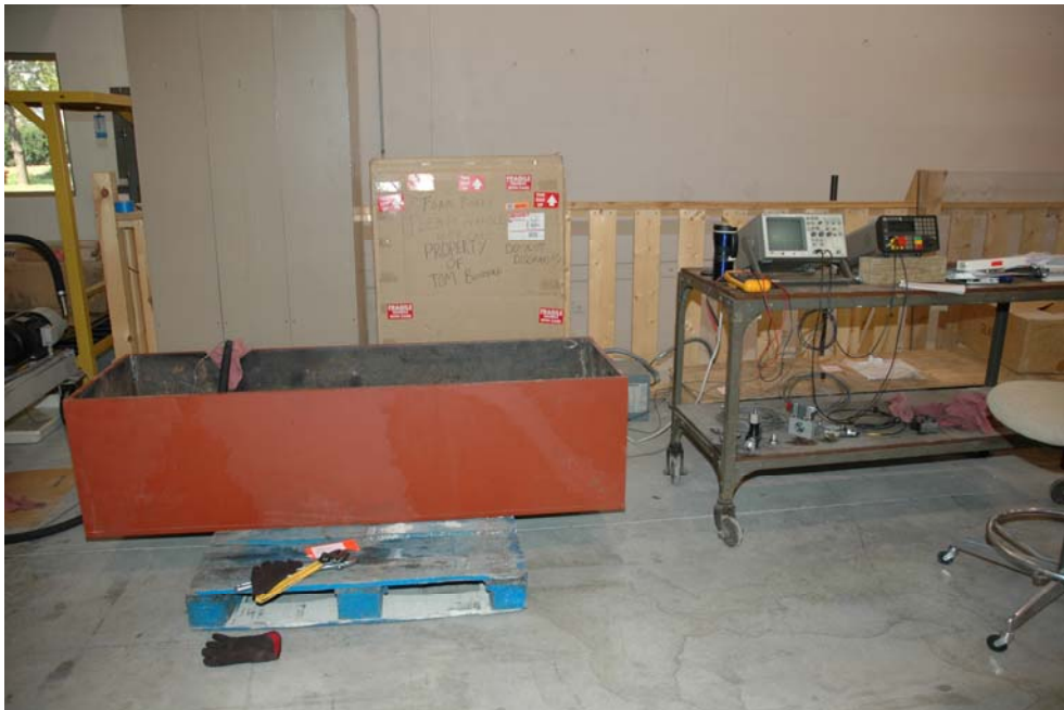
Figure 4: Test set up for pressure cycling test of DOT-3AA cylinder
