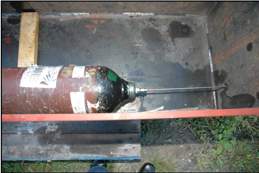
Figure 7: Test set up for hydraulic burst testing.
