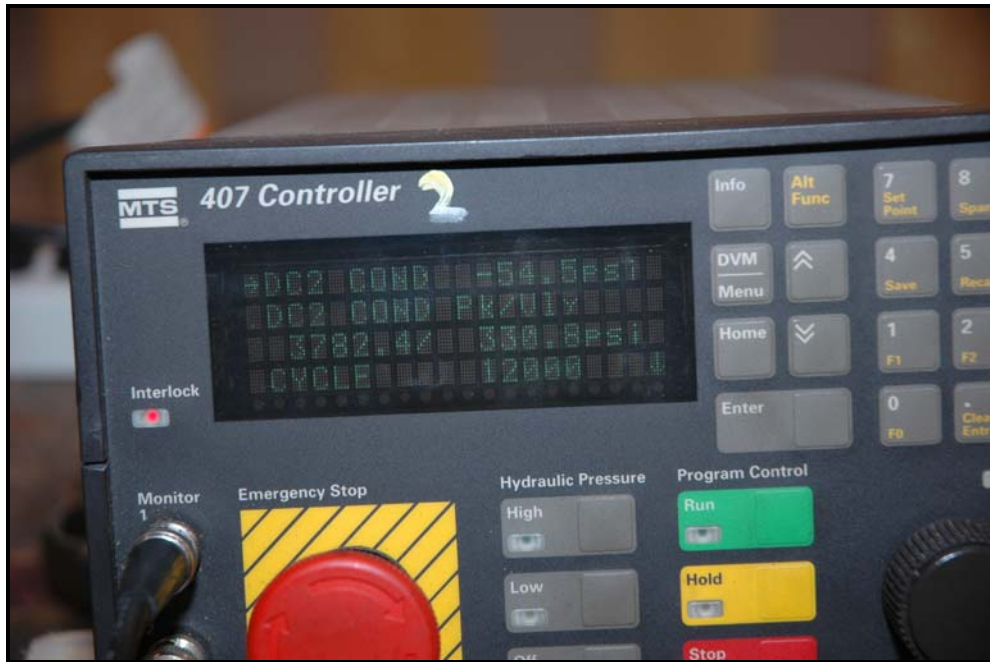
Figure 5: Shows the maximum/minimum pressure and cycles completed during cyclic testing of the DOT – 3AA cylinder.
