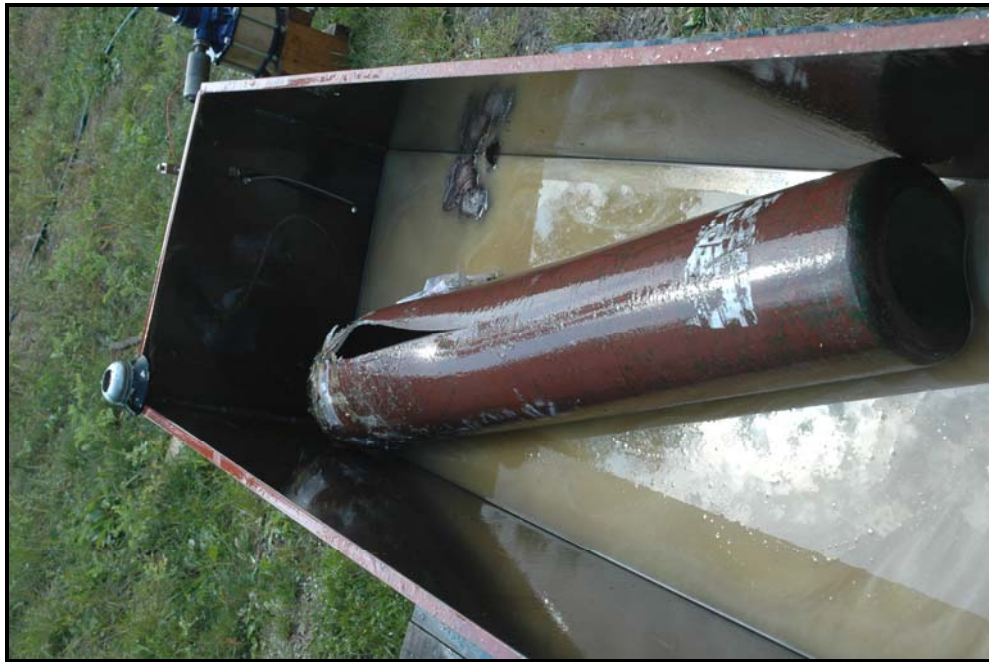
Figure 11: Ruptured cylinder after hydraulic burst testing.
