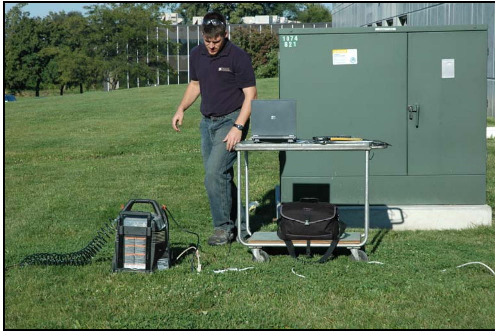
Figure 9: Test set up for hydraulic burst testing.
