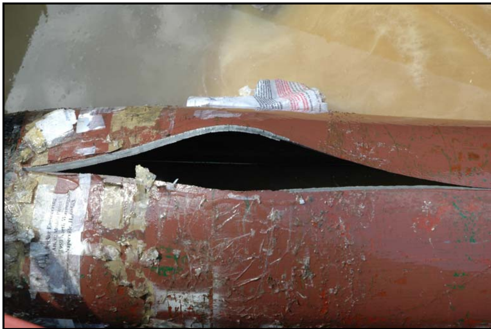
Figure 12: Ruptured cylinder after hydraulic burst testing.
