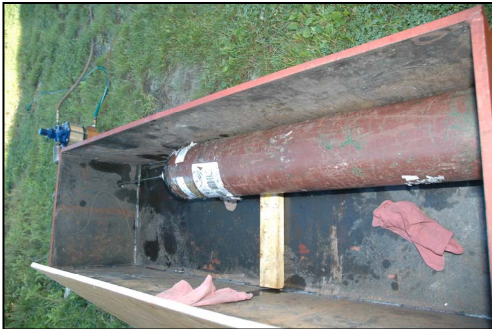
Figure 6: Test set up for hydraulic burst testing.
