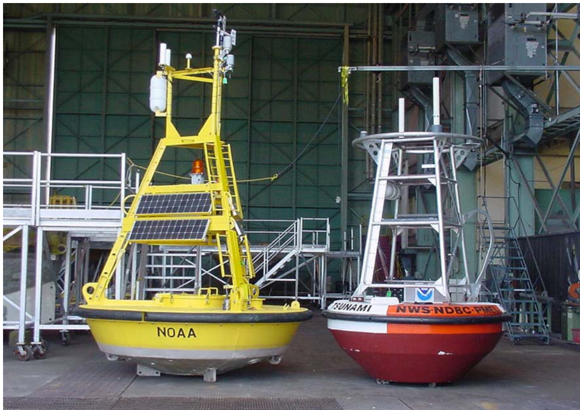
Figure 1: A Weather Buoy (left) and DART Buoy (right) in the NDBC Service Facility
