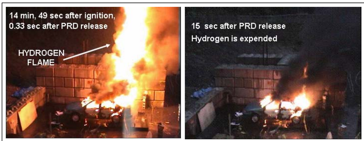
Figure 30. Hydrogen Vehicle Fire Showing Ignited Hydrogen Released from PRD
