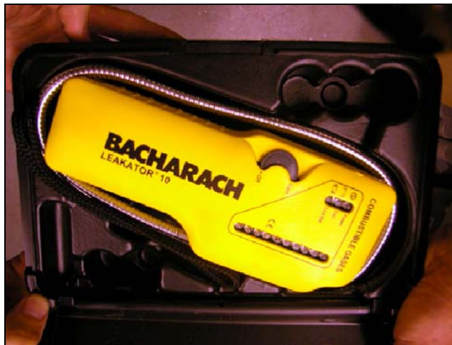
Figure 29. Hydrogen Leak Detector
