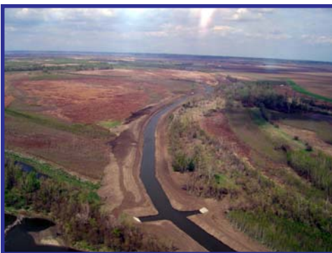
-USFWS This is an aerial view of the Lower Hamburg Bend chute on the Missouri River. It was constructed by the U.S. Army Corps of Engineers as part of the Missouri River Mitigation Program.
