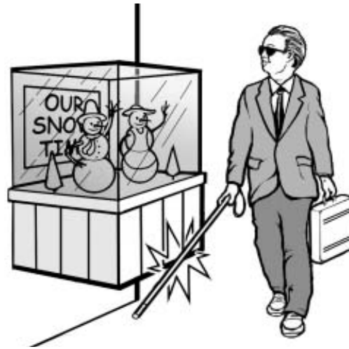
If the bottom of an object is not more than 27 above the floor, it may extend an unlimited amount from the wall.
