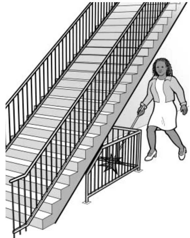
A detectable fence placed under this stair keeps people from running into the bottom of the open stair.
