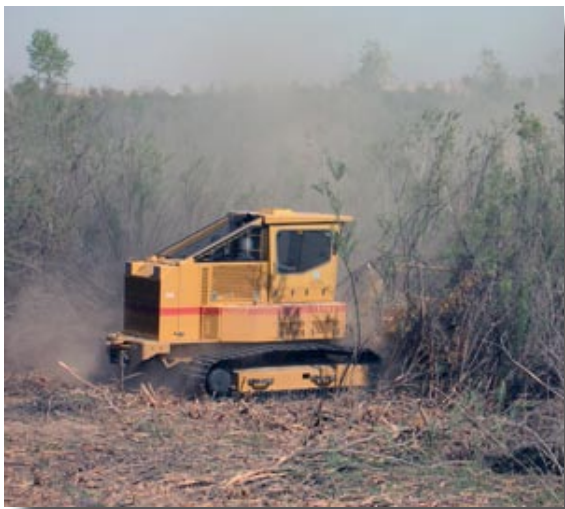
Fuel break treatment utilizing a bullhog.
