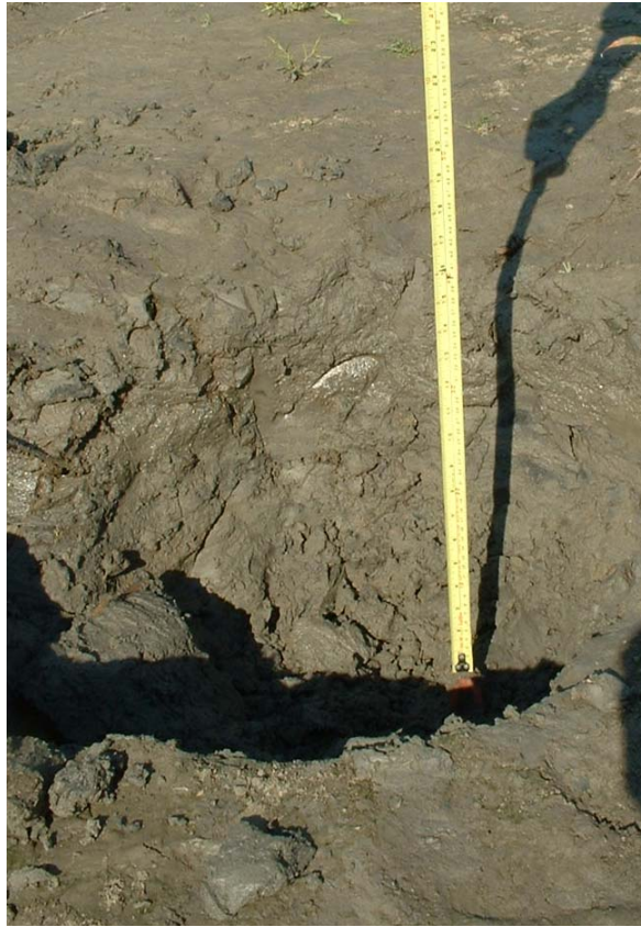
Figure B.3. Photographs documenting sediment deposition after a high flow event on sandbar Rkm 284 (mile 176.5b), surveyed on 07/28/2004.
