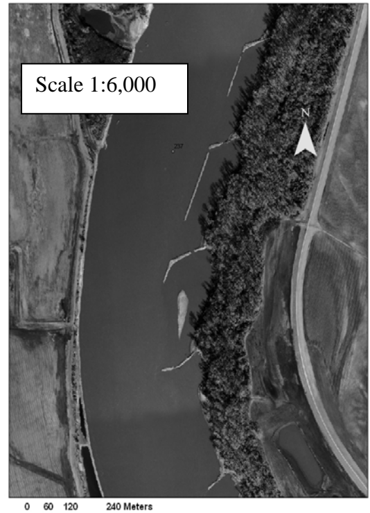
Figure 2.5. Representative elevation grids and orthophotographs for a point sandbar at km 253 (at 23 kcfs) and a wing-dike sandbar at km 381 (at 26 kcfs) within the Grand River to Osage River segment of the Missouri River, Missouri.
