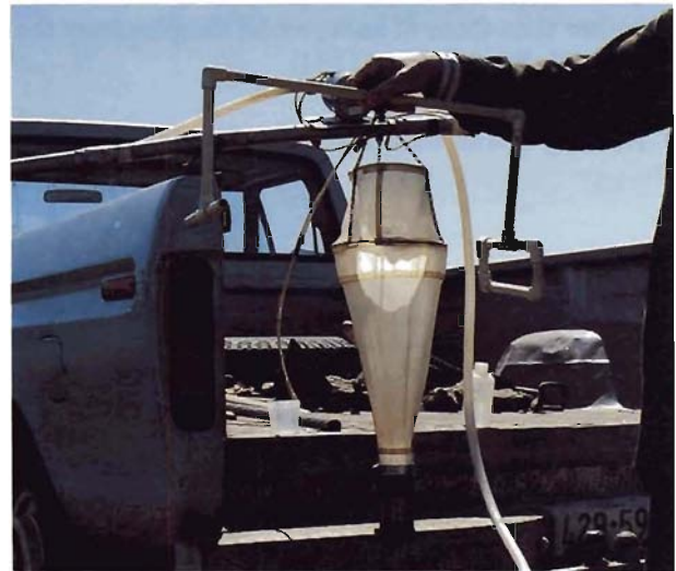
Top photo. Cladocerans such as Bosmina longirostris are highly sensitive to toxic substances. Their presence outside the affected area but absence in the kill zone is a valuable clue to the possible cause. Bottom photo. Plankton nets are used for collecting zooplankton to check for toxic effects.
