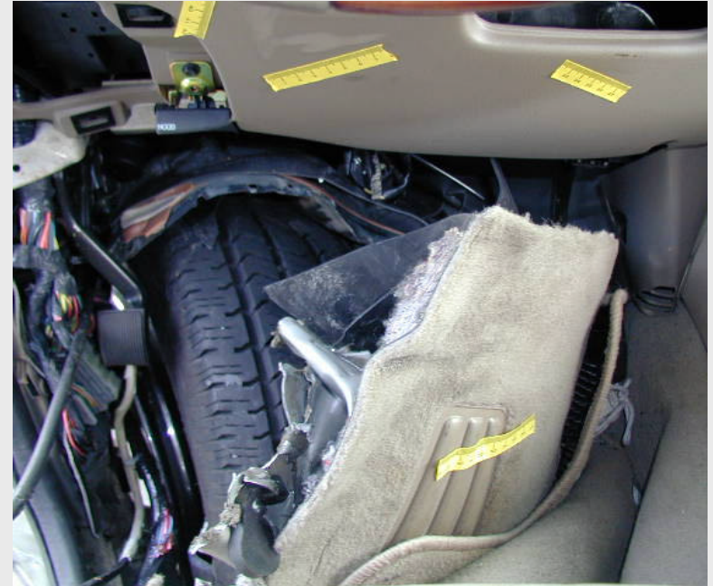
55 cm (21") longitudinal intrusion of toe pan
