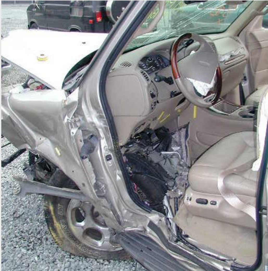
55 cm (21") longitudinal intrusion of toe pan
