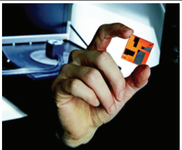
Figure 1.1: By blending ZnO nanoparticles and a conjugated polymer into a thin film, hybrid polymer solar cells can be made that give fourfold improved power conversion efficiency compared with that of existing hybrid solar cells based on metal oxides. Reference 2.
