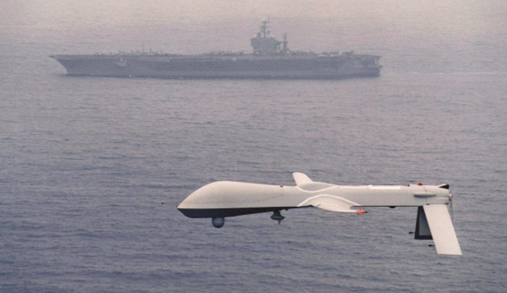
The Predator Unmanned Aerial Vehicle (UAV) flies above the USS Carl Vinton (CVN 70) on a simulated Navy reconnaissance flight headed by Command Carrier Group One about 100 miles off the San Diego coastline. Predator has a wingspan of 48.4 feet, a length of 26.7 feet and weighs approximately 1,500 pounds when fully fueled. Cost of the aircraft is around 3.2 million dollars. Average speed is approximately 70 knots. (U.S. Navy photo by PH3 Jeffrey S. Viano)
