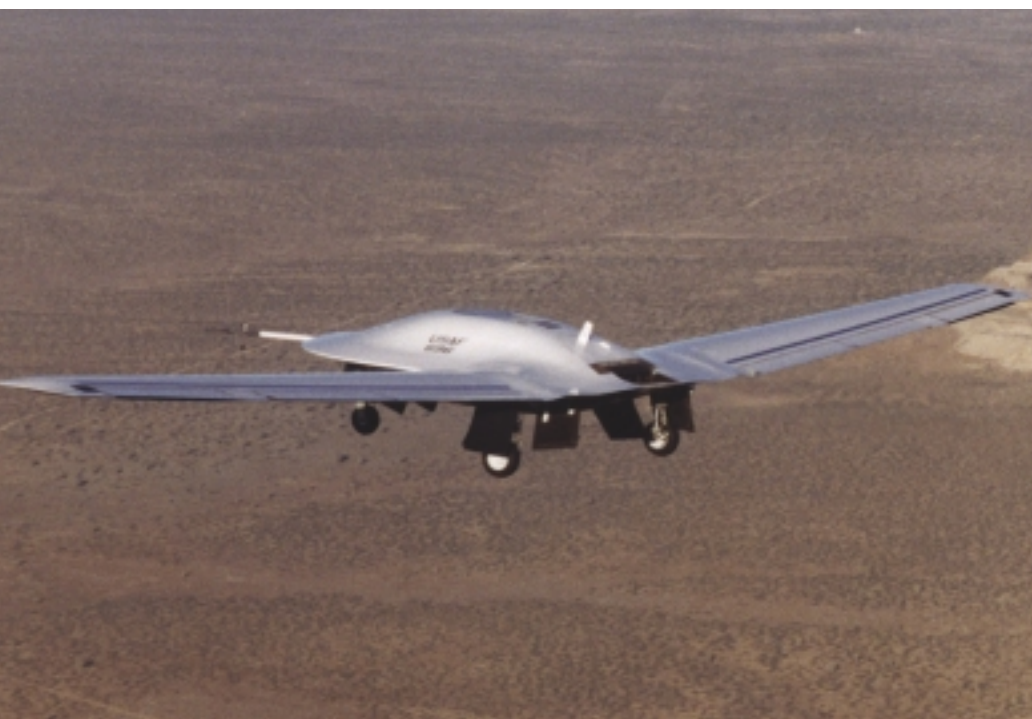
ABOVE: The new RQ-4A Global Hawk unmanned aerial vehicle flies through the sky during its maiden voyage here April 23. The Global Hawk is designed to provide battlefield commanders with near real-time, high-resolution, reconnaissance imagery. Flying at extremely high altitudes, Global Hawk can survey large geographic areas giving military decision-makers the most current information. (U.S. Air Force photo)
