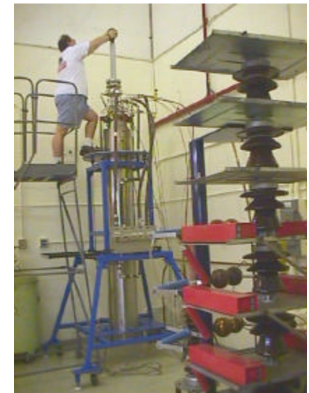
HV Impulse Generator and Large HV Cryostat
