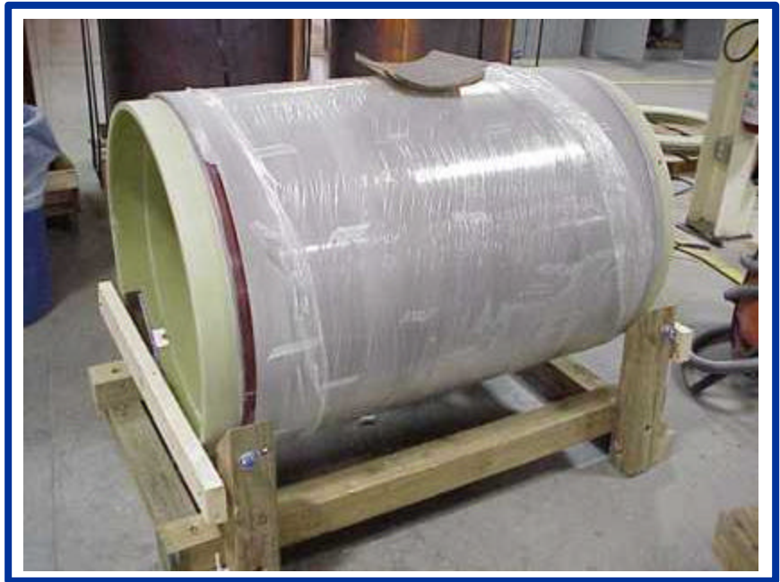
HV Coil Prepped for Phase Set Assembly
